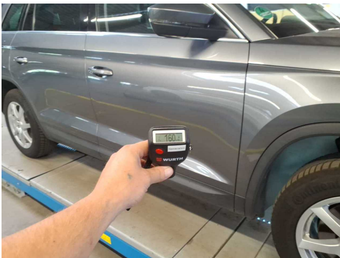
Repainting 4: Bumper front, Door - front right side
