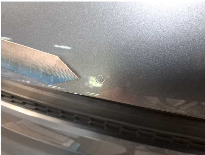
Damage 4: Boot lid / rear door: Boot lid (Rostpickel) - Paint defect - Smart repair
