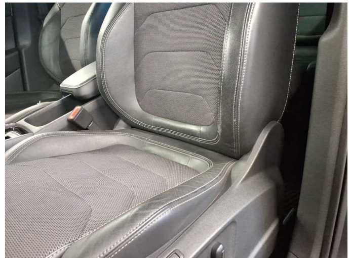
Damage 2: Seat - front: Seat cover - left side (Wange) - Abrasion - Smart repair
