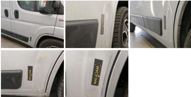
D-pillar right, Dent(s) and scratch(es), Repair and paint (complete)
