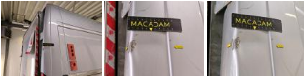
Bumper corner RR, Deformed / Strained, Replace and paint
