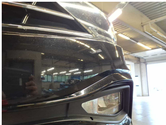
Damage 8: Front bumper: Front bumper (Sandstrahleffekt) - Stone chips - Paint
