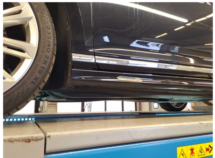
Damage 6: Sill - left side: Sill - Damaged - Smart repair
