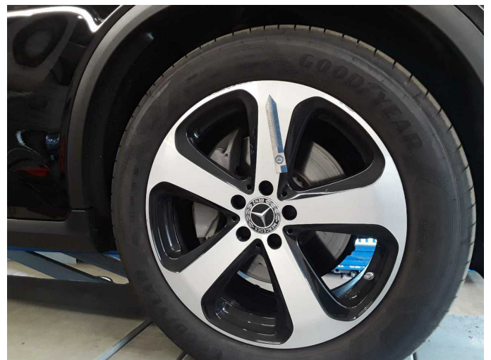
Damage 6: Wheel / tyres: Alloy rim - front right side (Materialabtrag) - Scratched - Replace
