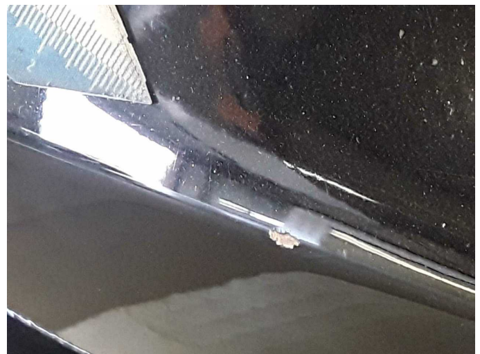
Damage 3: Boot lid / rear door: Boot lid - Corrosion - Smart repair
