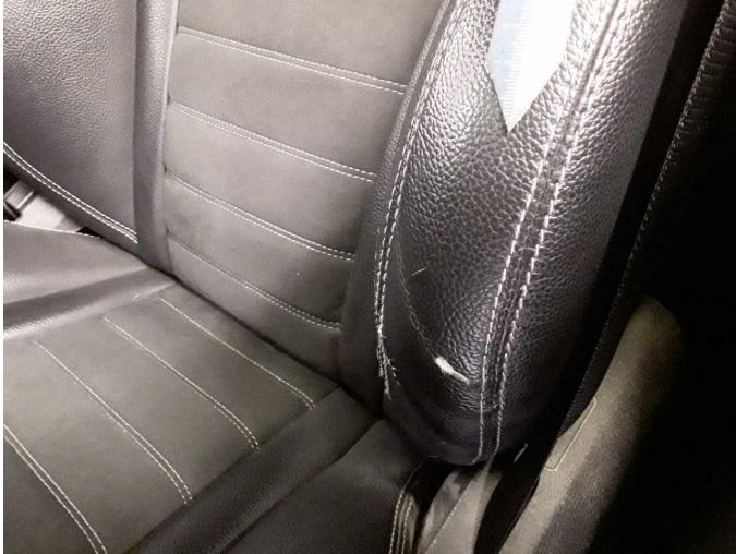
Damage 4: Seat - front: Backrest cover - left side - Damaged - Replace
