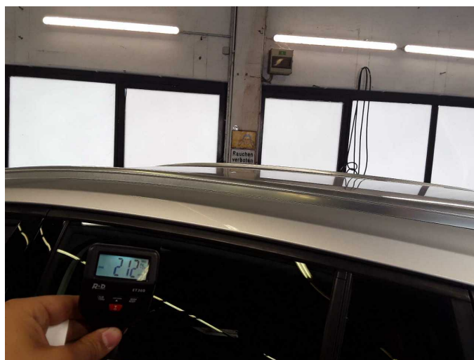
Roof rail - left side: 212 µm
