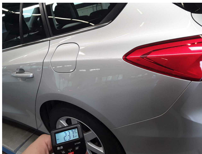
Side panel - rear left side: 237 µm
