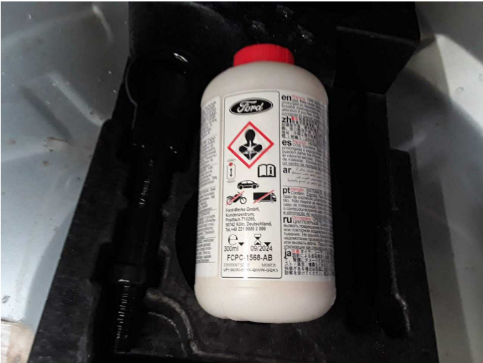
Damage 1: Equipment: Tirefit filler - Expired - Replace
