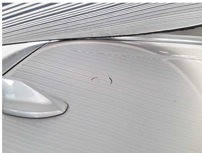
Damage 9: Roof: Roof - dent(s) - repair according to calculation
