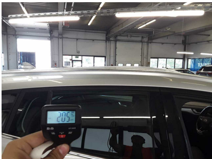
Roof rail - right side: 205 µm
