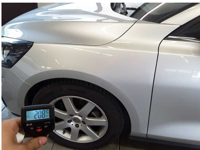
Mudguard - left side: 208 µm
