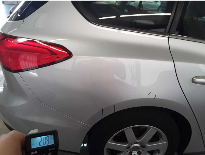
Side panel - rear right side: 209 µm
