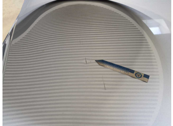
Damage 5: Bonnet: Bonnet - Dent / paintcoat damage - Paint
