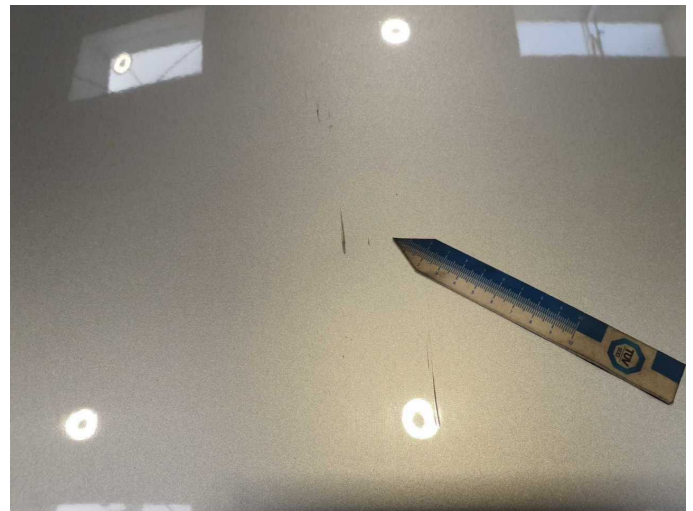
Damage 5: Bonnet: Bonnet - Dent / paintcoat damage - Paint
