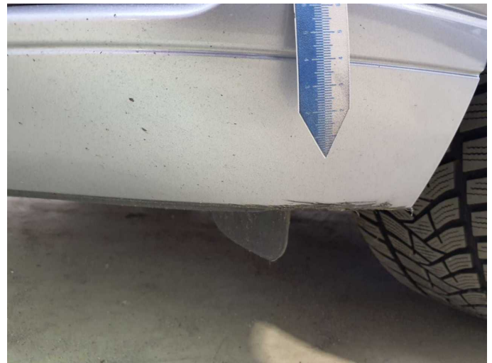
Damage 4: Front bumper: Front bumper - Scratch(es) - Paint
