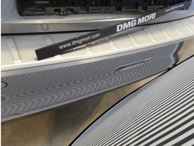
Damage 3: Rear bumper: Rear bumper - Dent / paintcoat damage - Paint
