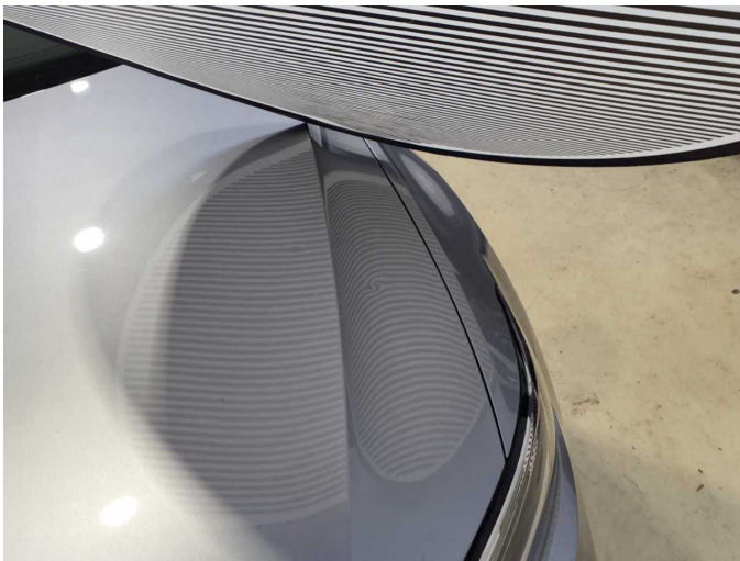
Damage 5: Bonnet: Bonnet - Dent / paintcoat damage - Paint
