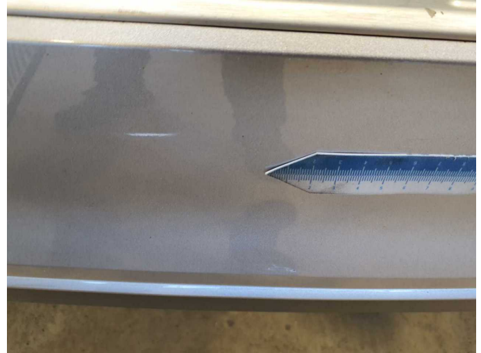
Damage 3: Rear bumper: Rear bumper - Dent / paintcoat damage - Paint
