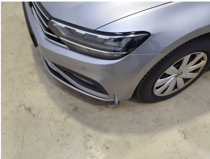
Damage 4: Front bumper: Front bumper - Scratch(es) - Paint
