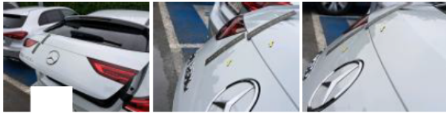
Rear light R tailgate, Broken, Replace
