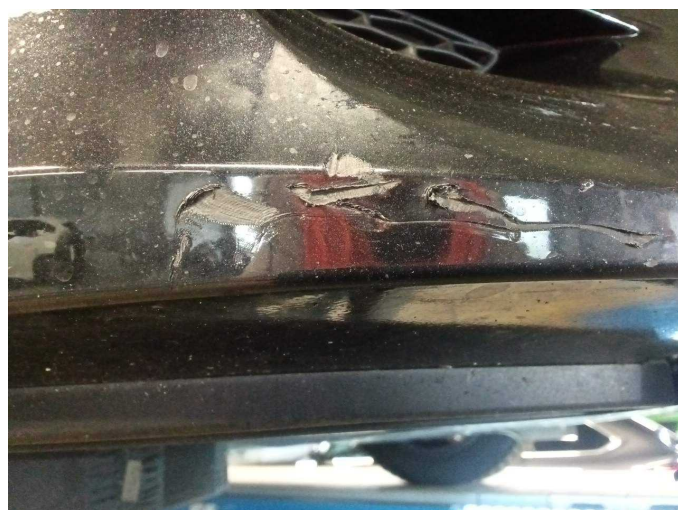
Damage 12: Front bumper: Front bumper - Broken / torn - Replace
