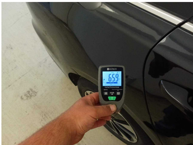
Side panel - rear right side: 659 µm
