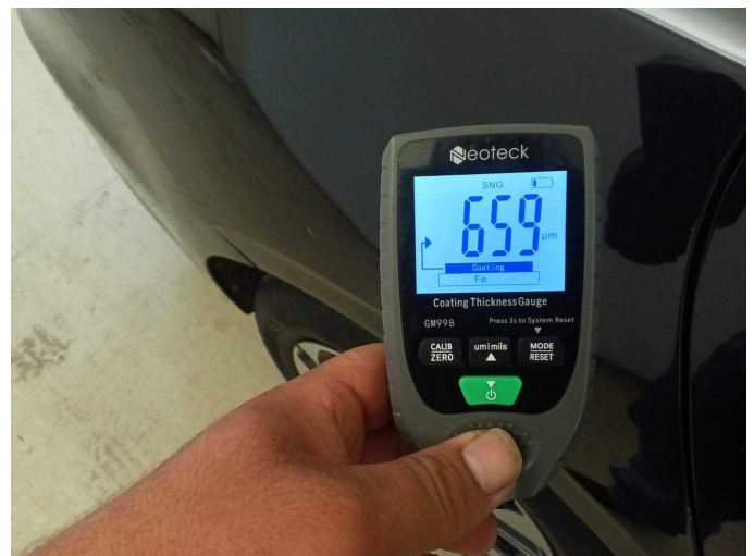
Side panel - rear right side: 659 µm
