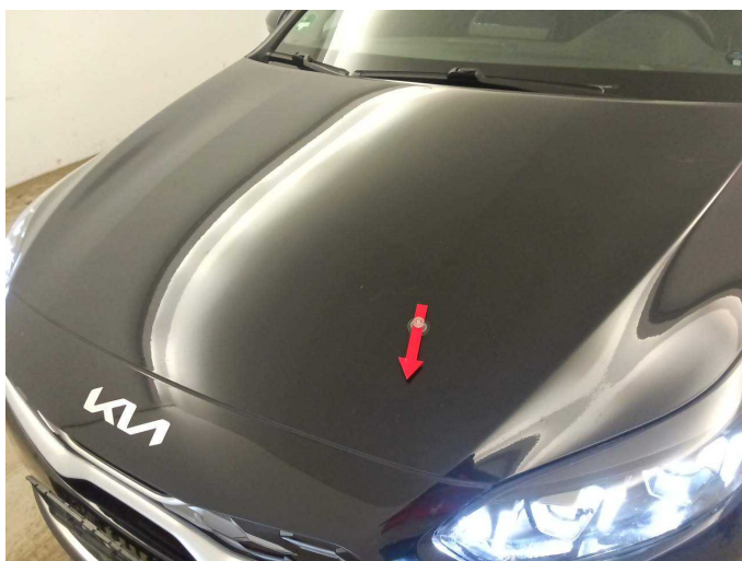
Damage 9: Bonnet: Bonnet - Stone chips - Paint
