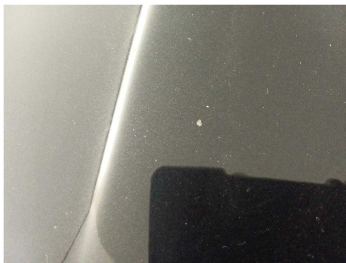
Damage 9: Bonnet: Bonnet - Stone chips - Paint
