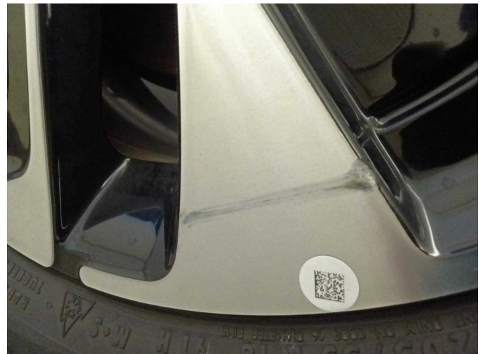
Damage 7: Wheel / tyres: Alloy rim - rear right side - Scratch(es) - Replace
