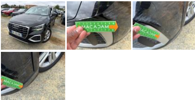
Bumper moulding FL, Scratch(es), Paint
