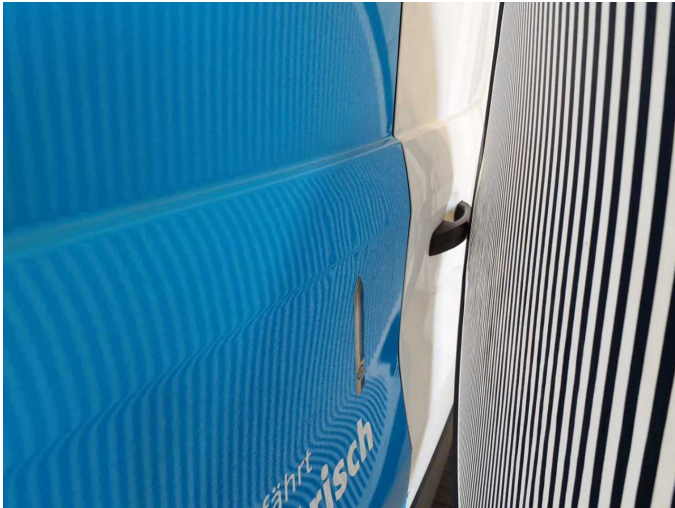
Damage 11: Boot lid / rear door: Rear door - left side - dent(s) - Smart repair
