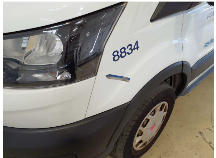
Damage 21: Mudguard - left side: Mudguard - left side - Dent / paintcoat damage - Repair and paint
