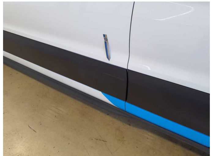
Damage 4: Side panel - rear left side: Brightware - Scratch(es) - Loss in value
