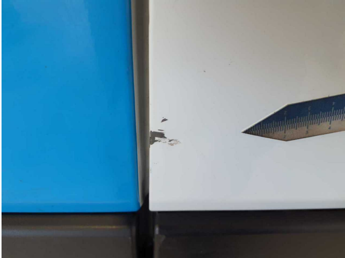
Damage 14: Boot lid / rear door: Rear door - right side - Dent / paintcoat damage - Smart repair
