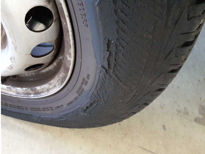
Damage 20: Wheel / tyres: Tyres - complete set (Und porös, nicht fahrbereit) - Does not meet the leasing specifications - Replace
