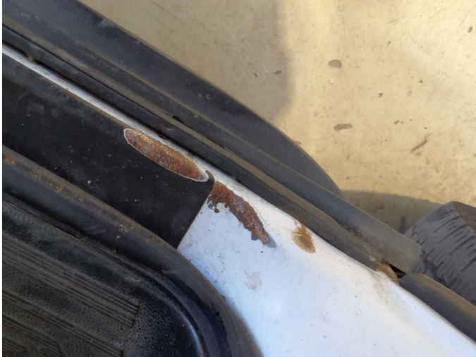
Damage 8: Sill - left side: Sill - Corrosion - Smart repair
