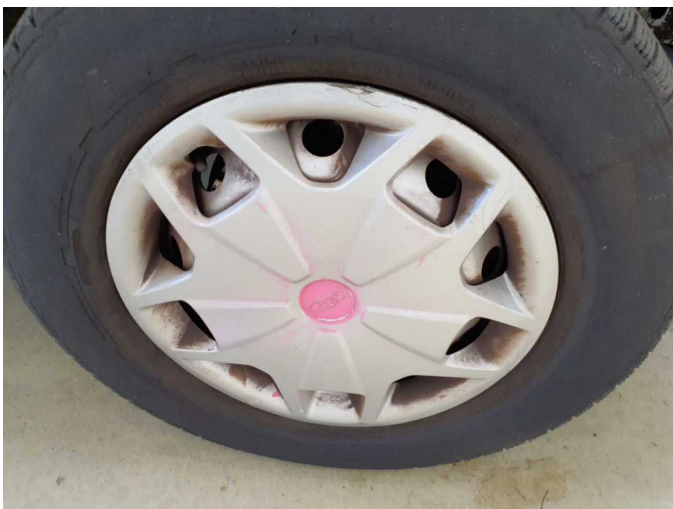
Wear and tear 4: Wheel / tyres: Wheel cover set - complete (3x) - Damaged - No deduction
