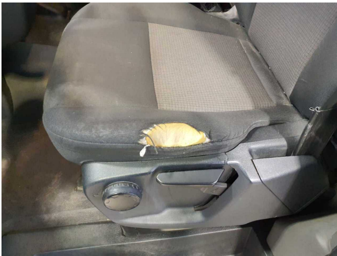
Damage 19: Seat - front: Seat cover - left side (+ Polster) - Broken / torn - Replace
