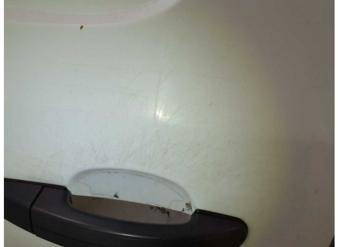
Wear and tear 5: Sliding door, right: Sliding door - Scratch(es) - Conditioning
