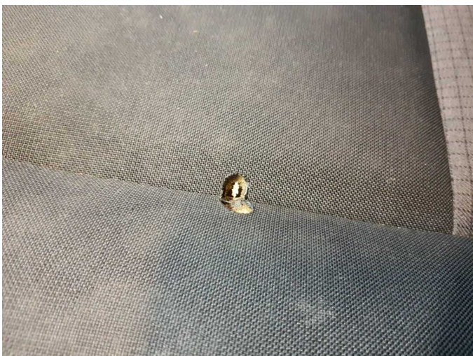
Damage 7: Seat - front: Seat cover - right side - Burn hole (cigarettes) - Smart repair
