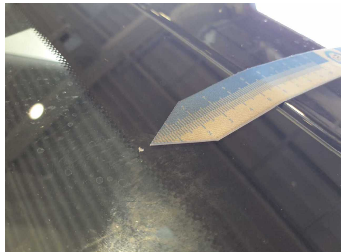
Damage 10: Vehicle glazing: Windscreen - Stone chips - Replace
