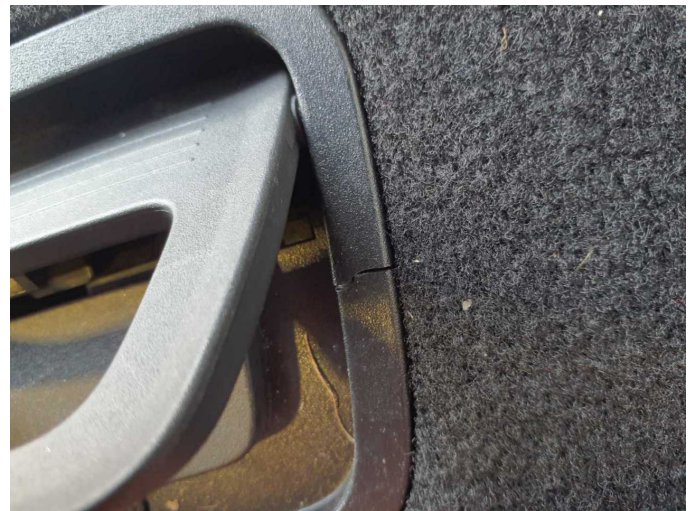
Damage 3: Interior: Cargo area floor (Griffabdeckung) - Broken / torn - Replace
