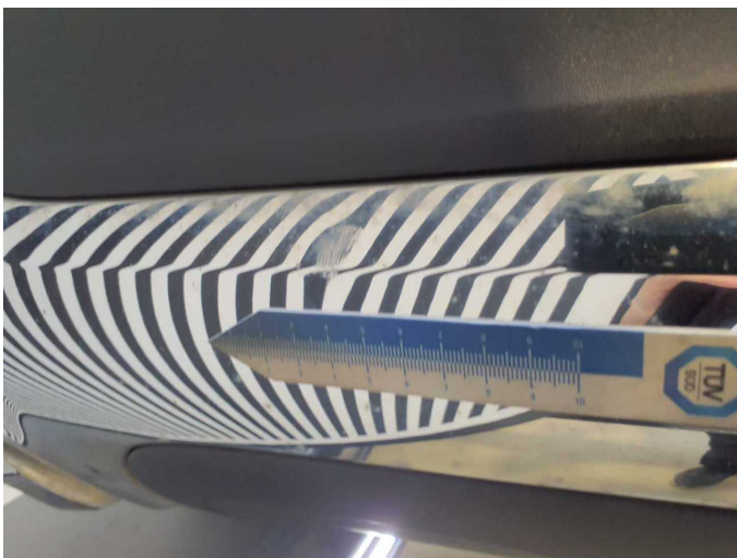
Damage 8: Rear bumper: Rear bumper (Zierleiste) - dent(s) - Replace
