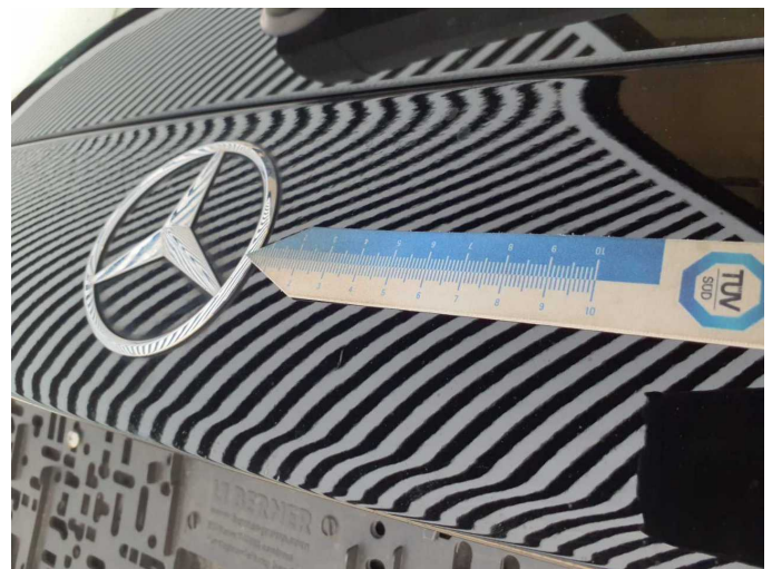
Damage 4: Boot lid / rear door: Boot lid - Dent / paintcoat damage - Smart repair
