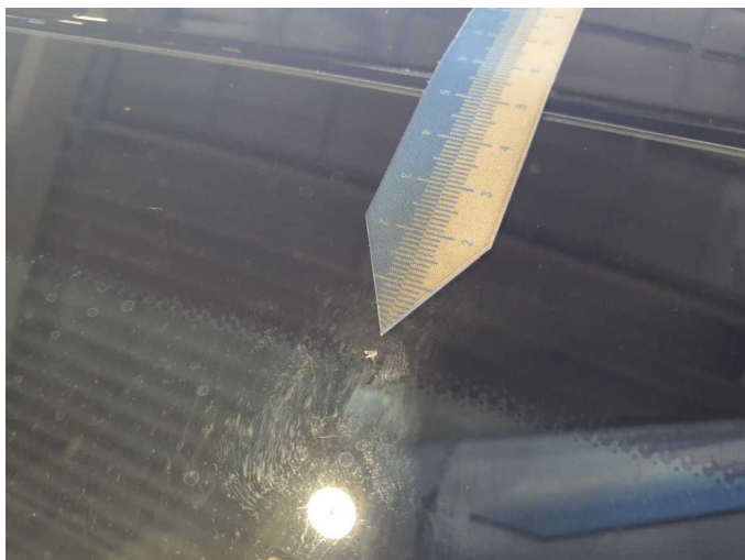
Damage 10: Vehicle glazing: Windscreen - Stone chips - Replace
