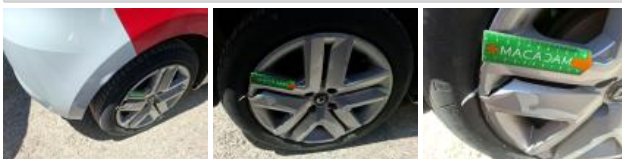
Tyre FR, Out of tolerance, Replace
