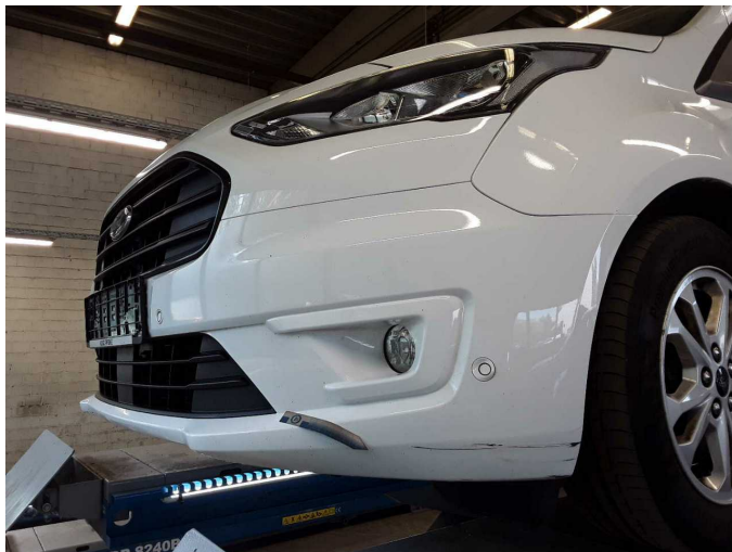
Damage 7: Front bumper: Front bumper - Scratch(es) - Paint
