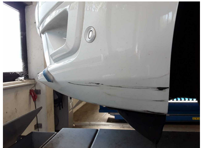
Damage 7: Front bumper: Front bumper - Scratch(es) - Paint
