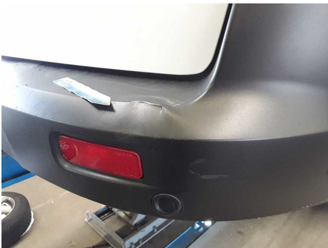
Damage 5: Rear bumper: Rear bumper (unpainted) - Deformed - Replace
