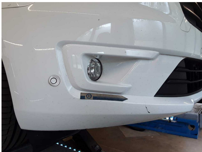
Damage 7: Front bumper: Front bumper - Scratch(es) - Paint
