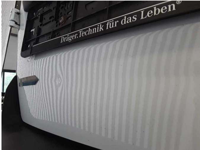
Damage 6: Boot lid / rear door: Rear door - left side - Deformed - Repair and paint
