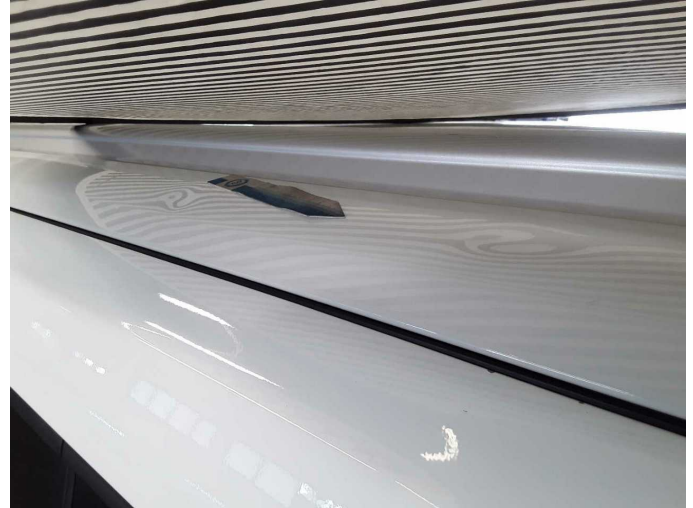
Damage 4: Roof: Roof rail - right side - dent(s) - Smart repair
