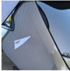
Damage Type Small dent(s)
