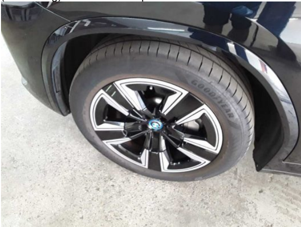
Damage #3: Wheel / tyres: Wheel cover - front left side (Abdeckung) - Scratched - Replace
