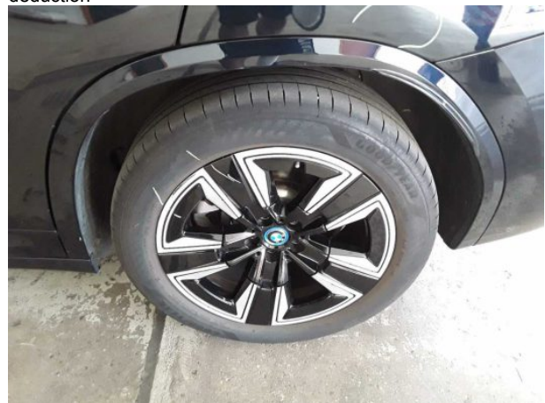
Damage #2: Wheel / tyres: Wheel cover - front left side (Abdeckung) - Scratched - Replace
