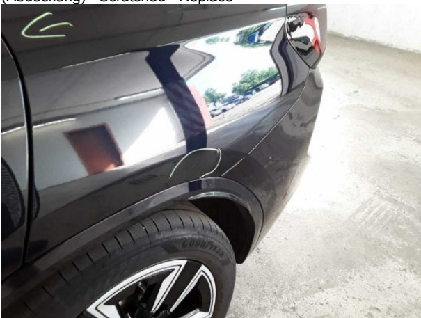
Damage #6: Side panel - rear left side: Side panel - Dent / paintcoat damage - Smart repair
