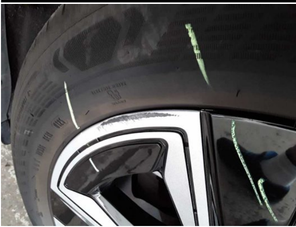
Damage #2: Wheel / tyres: Wheel cover - front left side (Abdeckung) - Scratched - Replace
