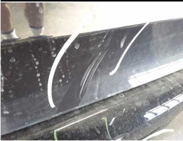
Damage #12: Boot lid / rear door: Boot lid - Scratched - Repair and paint
