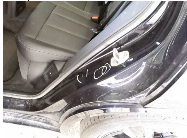
Damage #8: Side panel - rear left side: Sill - Dent / paintcoat damage - Repair and paint
