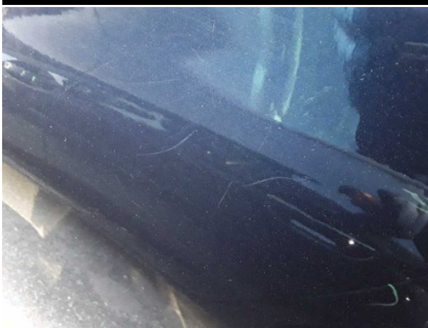
Damage #10: Door - rear left side: Door - Scratched - Repair and paint
