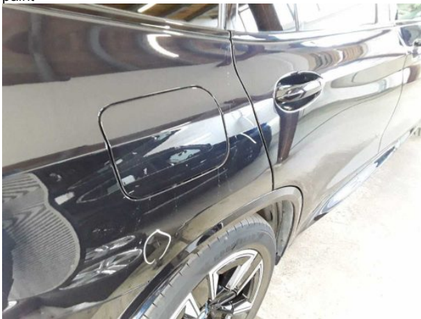
Damage #11: Side panel - rear right side: Side panel - Dent / paintcoat damage - Repair and paint
