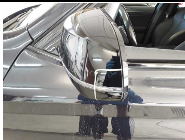
Damage #7: Wing mirror - left side: Mirror housing - Scratched... Smart repair
