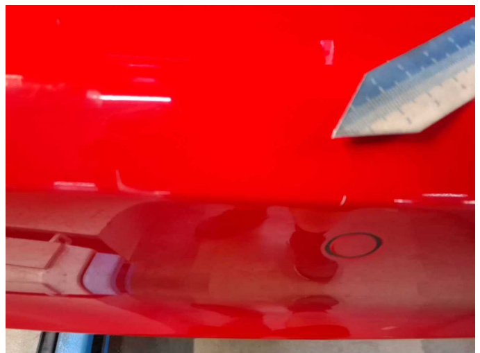
Damage 9: Rear bumper: Rear bumper - Scratched - Paint
