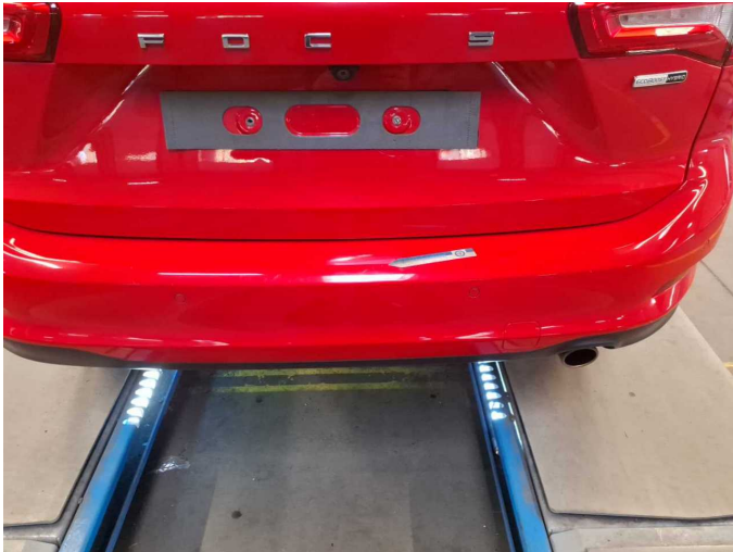
Damage 9: Rear bumper: Rear bumper - Scratched - Paint
