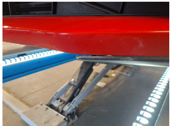
Damage 7: Front bumper: Spoiler - Damaged - Replace
