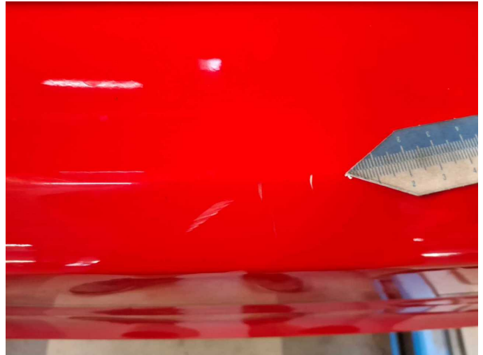
Damage 9: Rear bumper: Rear bumper - Scratched - Paint
