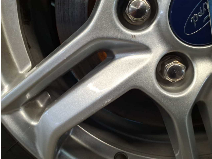
Damage 3: Wheel / tyres: Alloy rim - rear left side - Scratched - Smart repair
