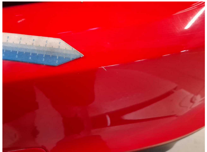
Damage 9: Rear bumper: Rear bumper - Scratched - Paint
