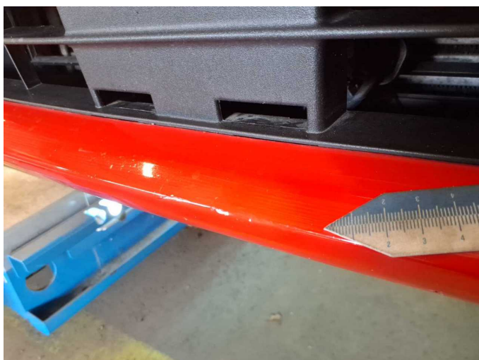
Damage 10: Front bumper: Front bumper - Damaged - Paint
