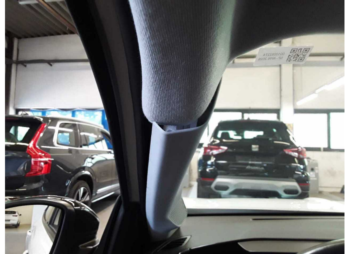
Damage 2: Trim / covers: A-pillar - trim - interior, left side - Damaged - Replace
