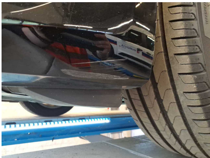
Damage 1: Front bumper: Front bumper - Scratch(es) - Paint
