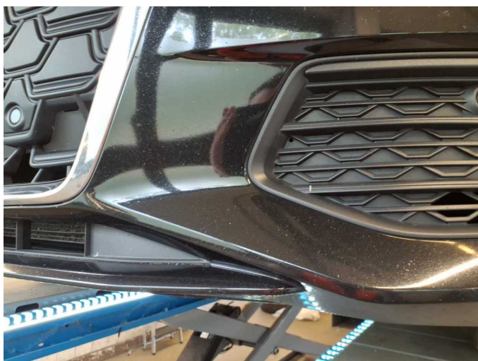
Damage 1: Front bumper: Front bumper - Scratch(es) - Paint
