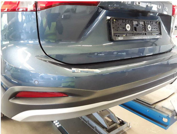
Damage 4: Rear bumper: Rear bumper - Scratch(es) - Paint
