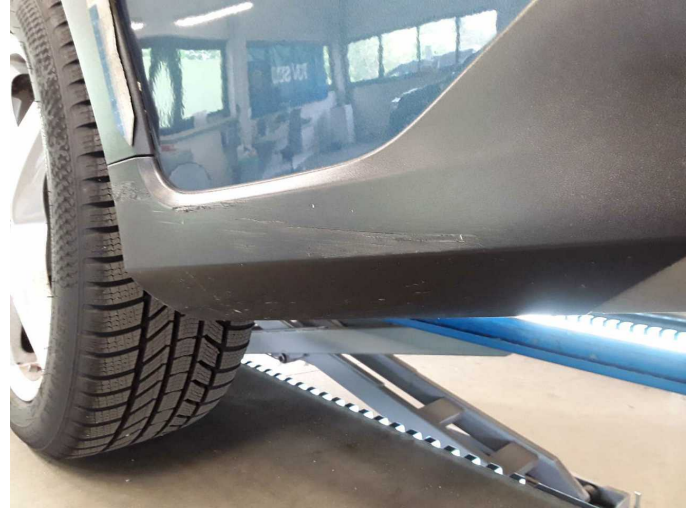
Damage 3: Rear bumper: Spoiler - Scratched - Replace
