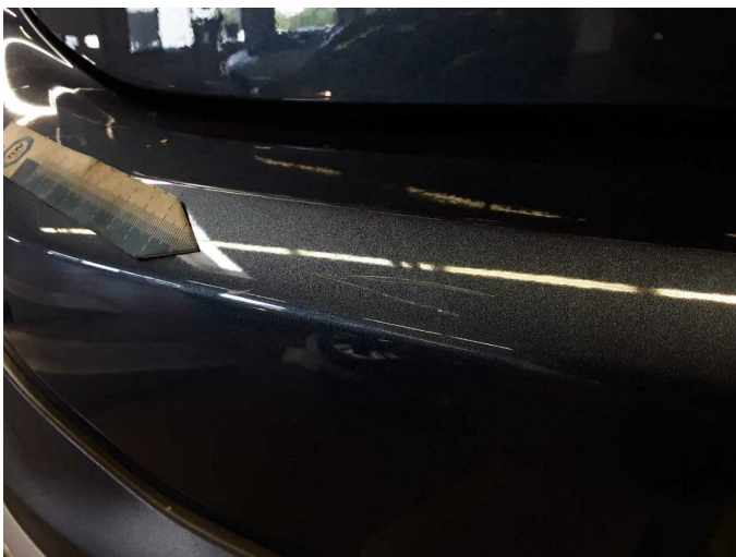
Damage 4: Rear bumper: Rear bumper - Scratch(es) - Paint
