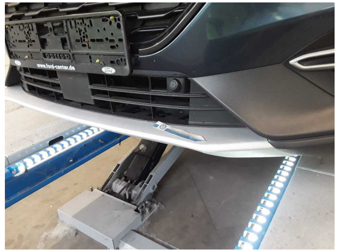
Damage 1: Front bumper: Spoiler - Scratched - Smart repair
