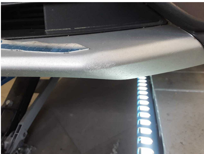
Damage 1: Front bumper: Spoiler - Scratched - Smart repair
