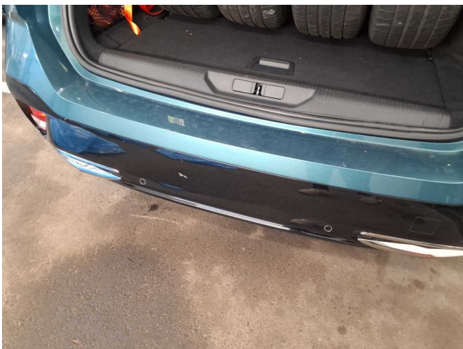
Damage 3: Rear bumper: Spoiler - Scratched - Replace
