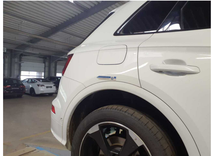
Damage 3: Side panel - rear right side: Side panel - dent(s) - Smooth repair work
