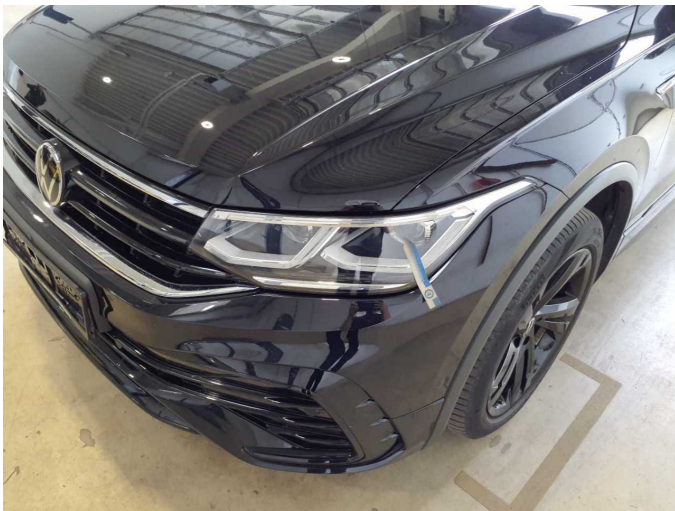
Damage 16: Headlight: Headlight - left side - Scratch(es) - Replace
