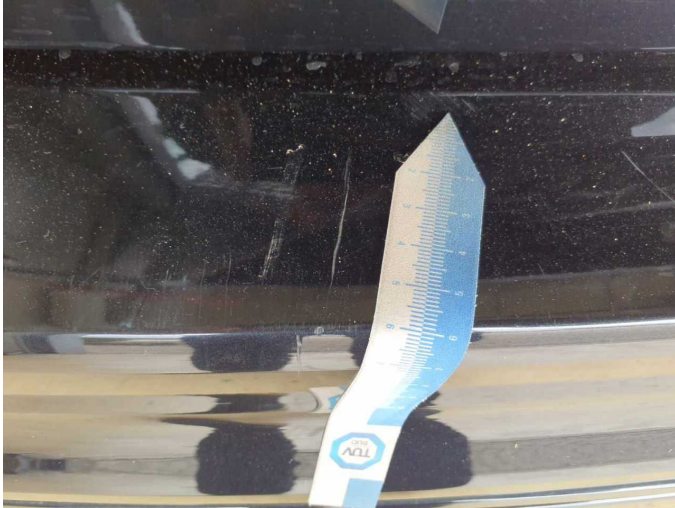
Damage 12: Rear bumper: Rear bumper - Scratch(es) - Paint
