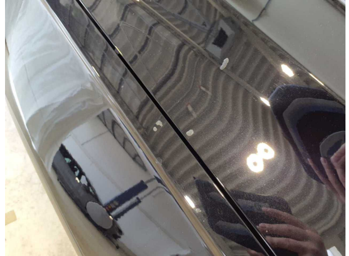
Damage 8: Body: Body (Harz) - Soiled - Conditioning
