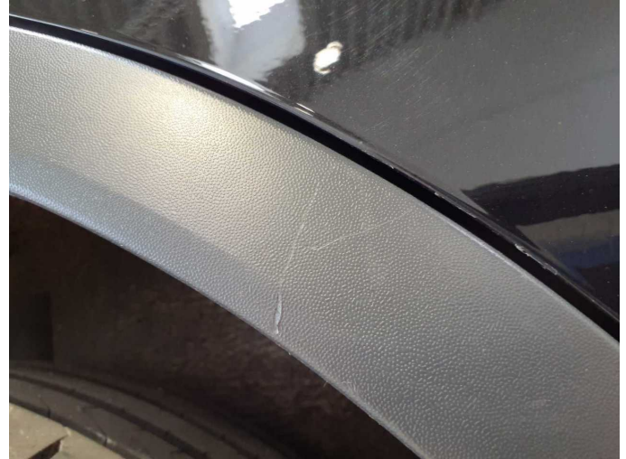
Damage 3: Side panel - rear right side: Wheel well extension - Scratch(es) - Loss in value
