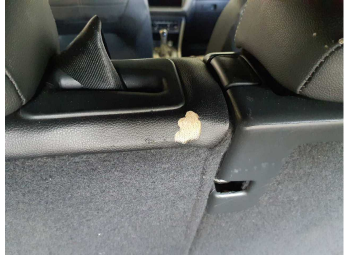
Damage 15: Seat - rear: Backrest cover - Broken / torn - Replace
