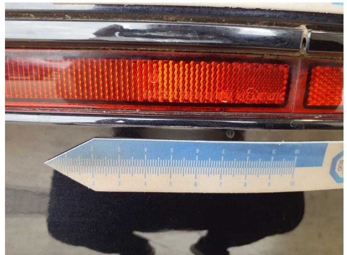
Damage 12: Rear bumper: Rear bumper - Scratch(es) - Paint
