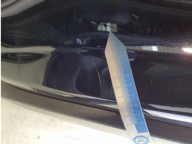
Damage 6: Side panel - rear left side: Sill - Scratch(es) - Smart repair
