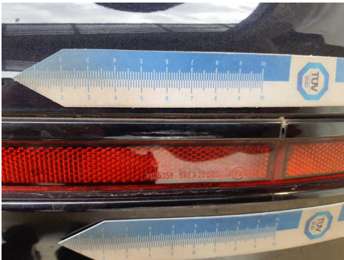
Damage 12: Rear bumper: Rear bumper - Scratch(es) - Paint
