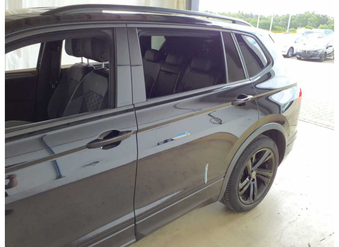
Damage 14: Door - rear left side: Door - Deformed - Repair and paint
