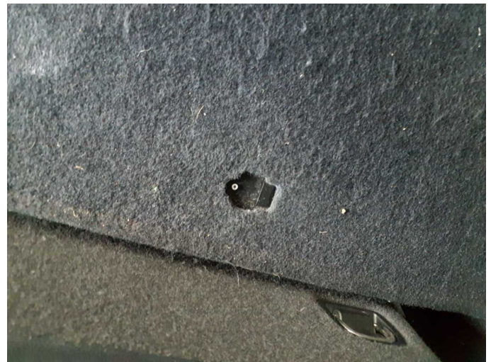
Damage 4: Seat - rear: Backrest cover - 2nd row (Griffband) - Missing - Replace
