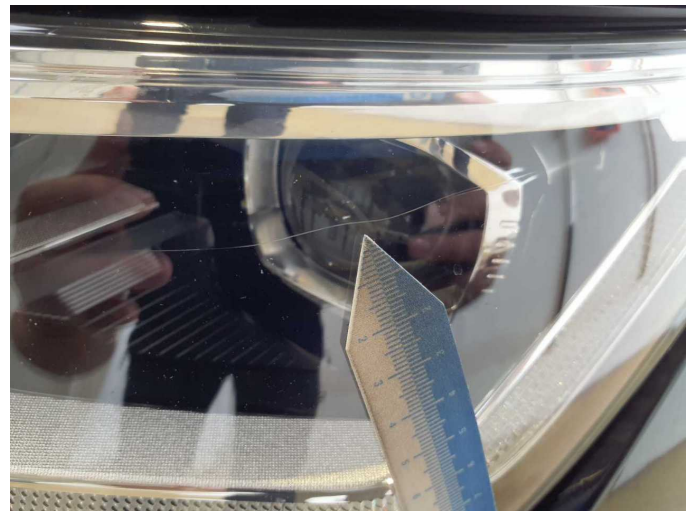
Damage 16: Headlight: Headlight - left side - Scratch(es) - Replace
