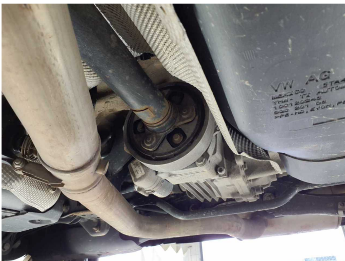
Damage 9: Drive train: Drive train (Hardyscheibe) - Porous / cracked - Replace
