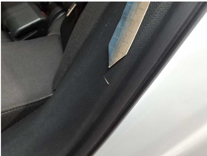
Damage 1: Side panel - rear left side: Interior trim - Scratch(es) - Loss in value
