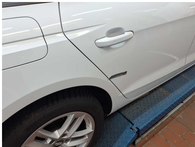
Damage 3: Side panel - rear right side: Elbow - dent(s) - Smart repair
