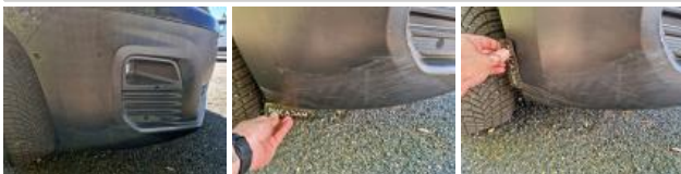
Wing FR, Dent(s), Repair and paint (complete)
