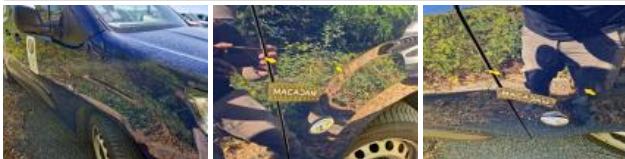
Door FR, Dent(s), Repair and paint (complete)
