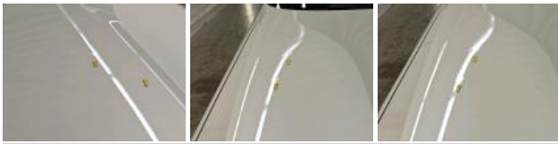
Windscreen, Stone chip(s), Windscreen repair
