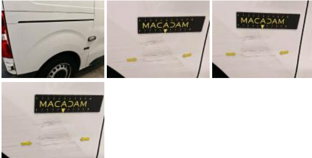
Sliding door R, Scratch(es), Repair and paint (complete)
