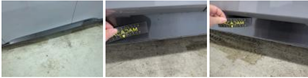
Bumper F, Crack, Repair and paint (complete)
