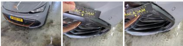
Bumper spoiler F, Broken, Replace
