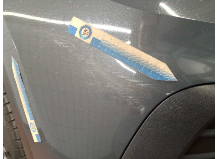
Damage 9: Front bumper: Front bumper - Scratched - Paint
