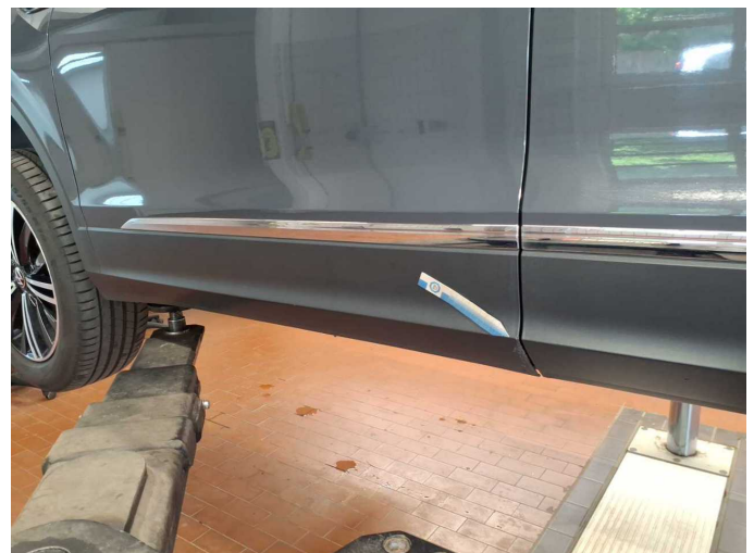
Damage 6: Door - front left side: Brightware - lower - Scratch(es) - Replace
