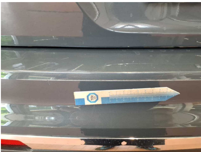
Damage 8: Rear bumper: Rear bumper - Scratch(es) - Paint
