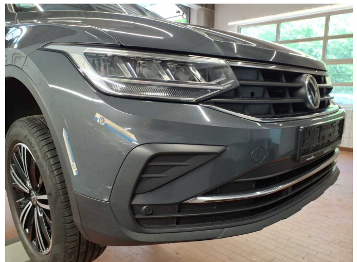
Damage 9: Front bumper: Front bumper - Scratched - Paint
