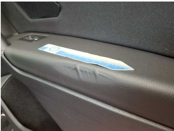
Damage 5: Trim / covers: Door trim - rear right side - Deformed - Loss in value
