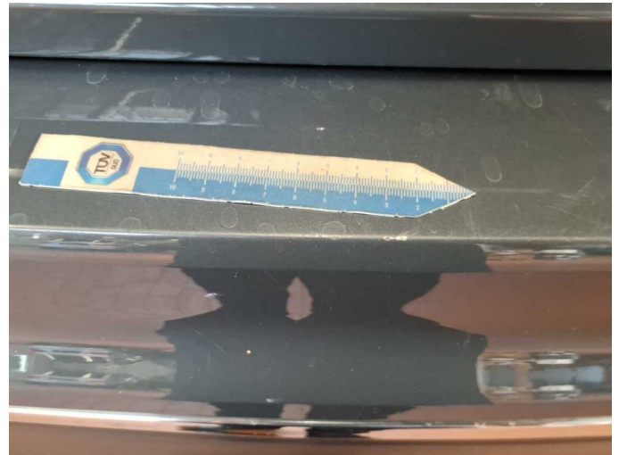
Damage 8: Rear bumper: Rear bumper - Scratch(es) - Paint
