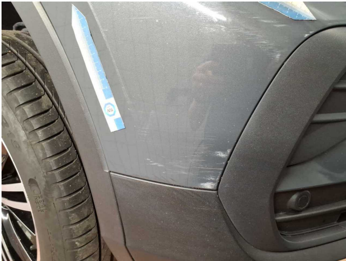
Damage 9: Front bumper: Front bumper - Scratched - Paint
