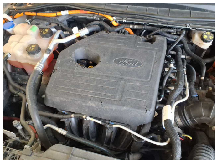
Damage 6: Engine: Engine cover - Damage caused by marten / rodent - Replace
