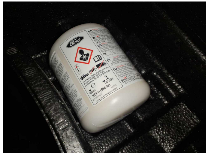
Damage 1: Equipment: Tirefit filler - Expired - Replace
