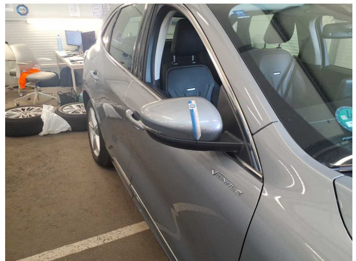
Damage 8: Wing mirror - right side: Mirror housing - Scratch(es) - Replace
