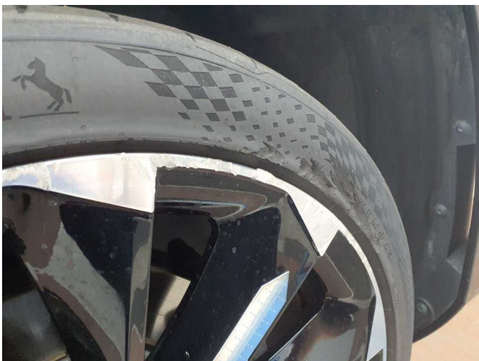
Damage 7: Wheel / tyres: Alloy rim - front right side (Materialabtrag) - Scratch(es) - Replace
