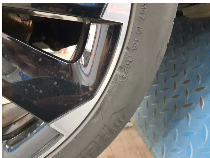
Damage 4: Wheel / tyres: Tyre - rear right side (nicht fahrbereit) - Damaged - Replace
