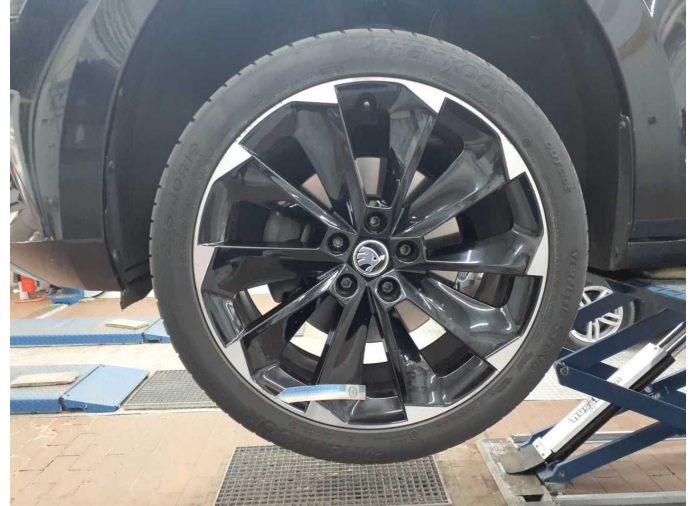
Damage 6: Wheel / tyres: Alloy rim - front left side (Materialabtrag) - Scratch(es) - Replace
