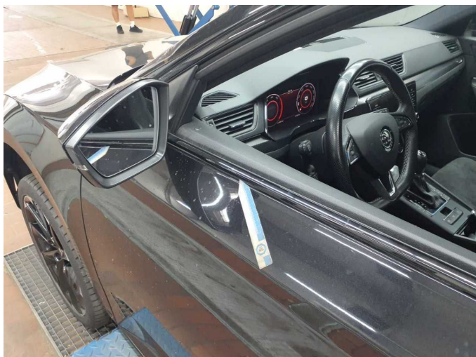
Damage 3: Door - front left side: Brightware - upper - Scratched - Replace
