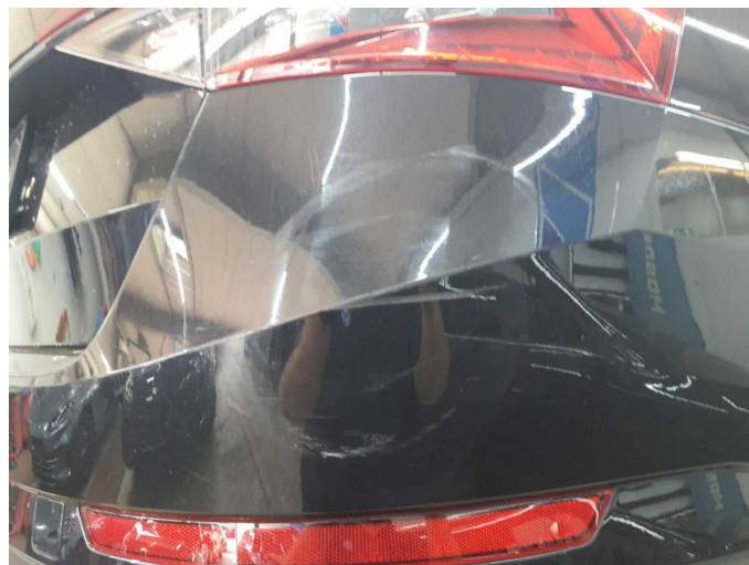
Damage 8: Rear bumper: Rear bumper - Scratch(es) - Paint
