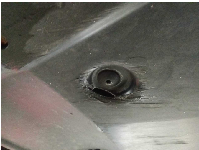
Damage 5: Body: Underbody panelling - Scratched - Replace
