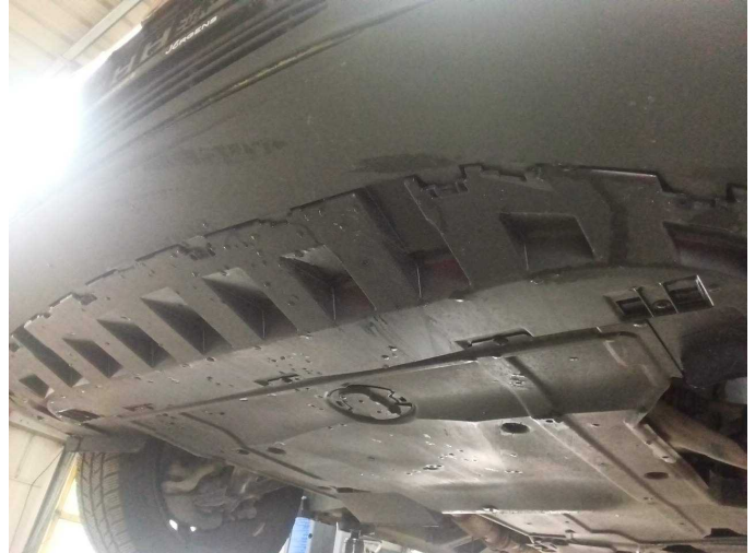
Damage 5: Body: Underbody panelling - Scratched - Replace
