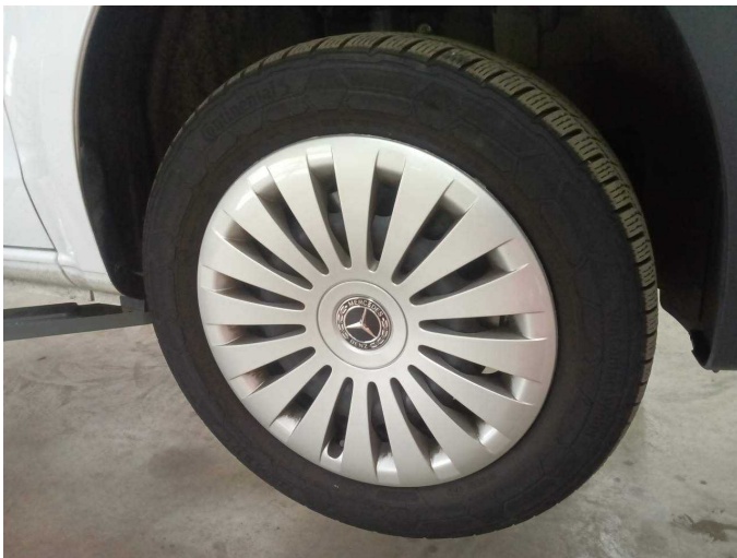
Damage 3: Wheel / tyres: Tyre - front right side - Porous / cracked - Replace
