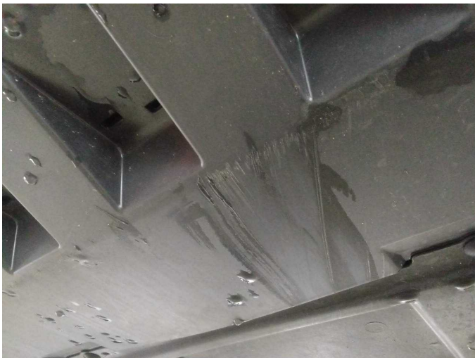
Damage 5: Body: Underbody panelling - Scratched - Replace
