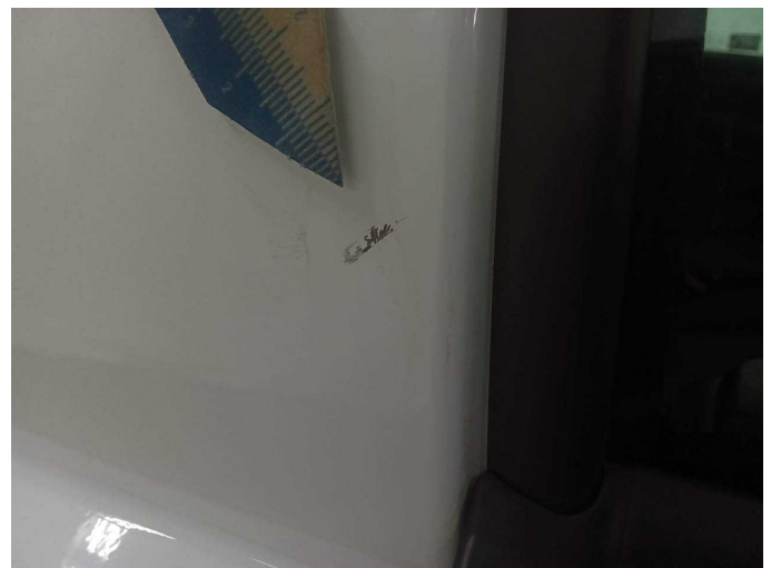
Damage 4: Door - front right side: Door - Dent / paintcoat damage - Smart repair
