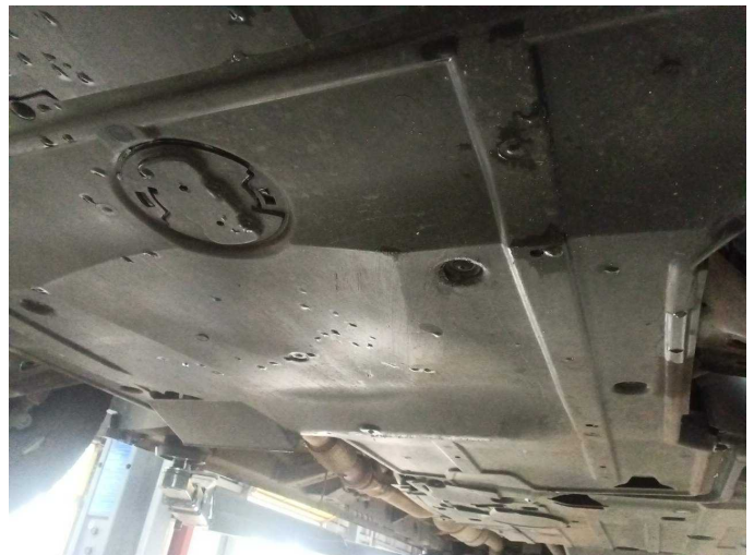
Damage 5: Body: Underbody panelling - Scratched - Replace
