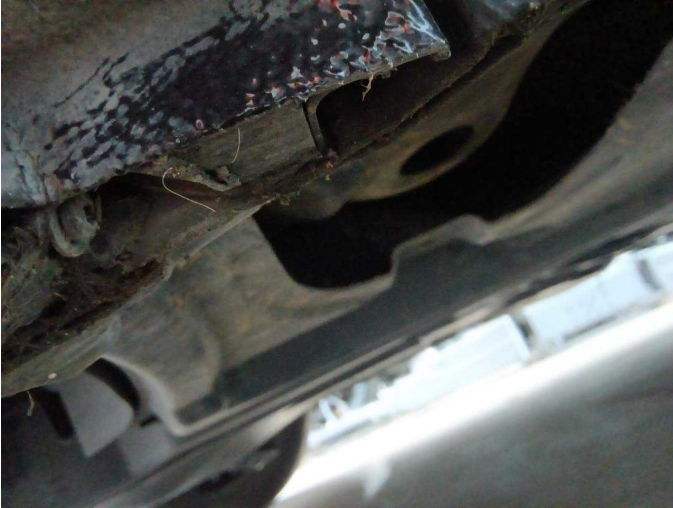
Damage 2: Sill - left side: Jacking point - front - Missing - Replace
