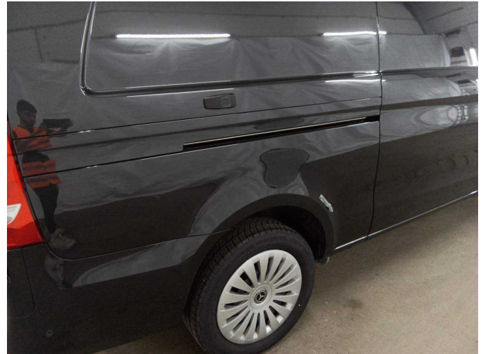
Damage 4: Side panel - rear right side: Mudguard - rear right side - Stone chips - Smart repair
