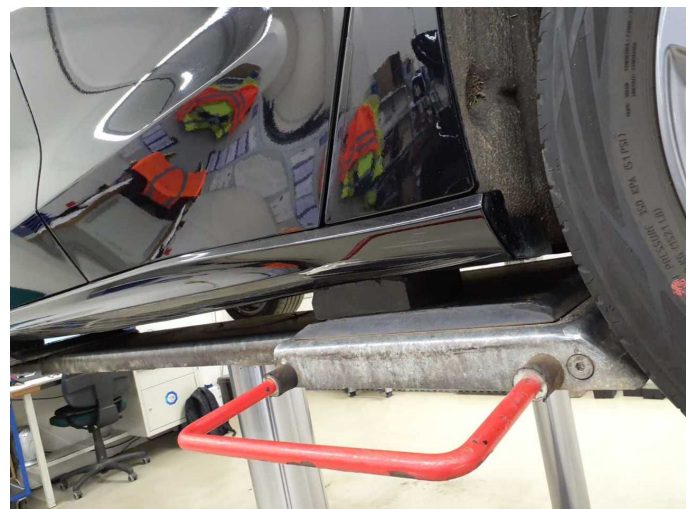
Damage 6: Sill - left side: Trim - Scratched - Paint
