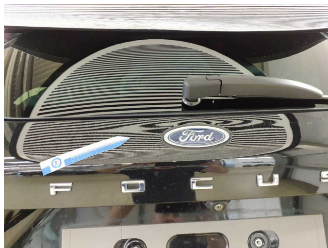
Damage 9: Boot lid / rear door: Boot lid - Dent / paintcoat damage - Repair and paint
