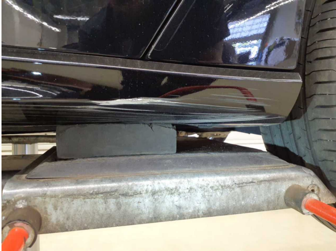
Damage 6: Sill - left side: Trim - Scratched - Paint
