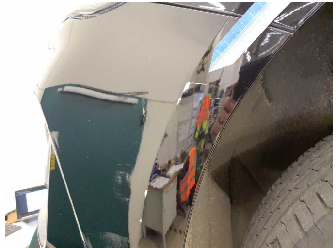
Damage 7: Front bumper: Bumper with Parktronic - Scratched - Paint
