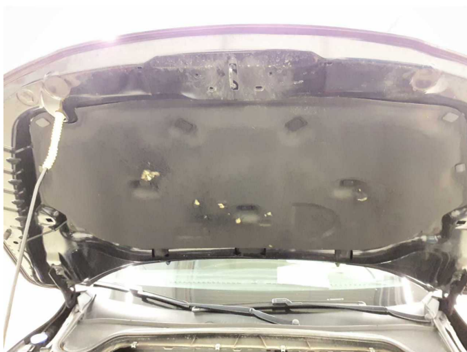
Damage 1: Bonnet: Insulation lining - Broken / torn - Replace
