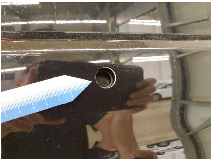
Damage 10: Rear bumper: Bumper with Parktronic - Deformed - Replace
