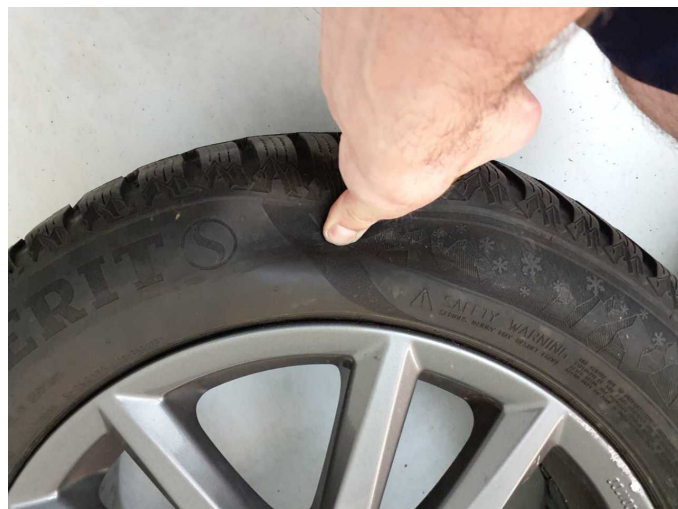
Damage 2: 2nd wheel set: 1 tyre - Defective - Replace
