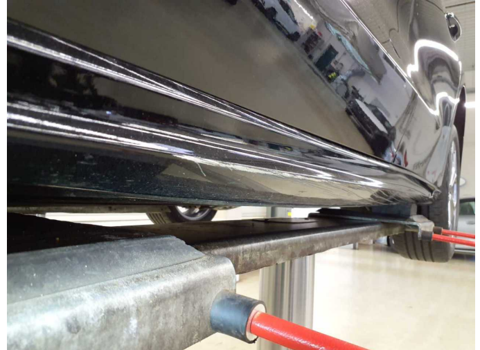
Damage 6: Sill - left side: Trim - Scratched - Paint
