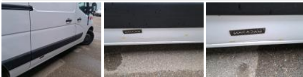
Outer sill R, Scratch(es), Paint
