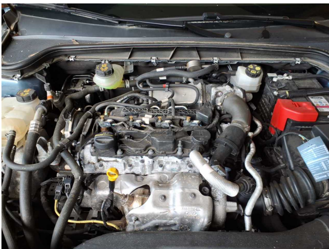
Missing part 2: Engine: Engine cover - Missing - Replace
