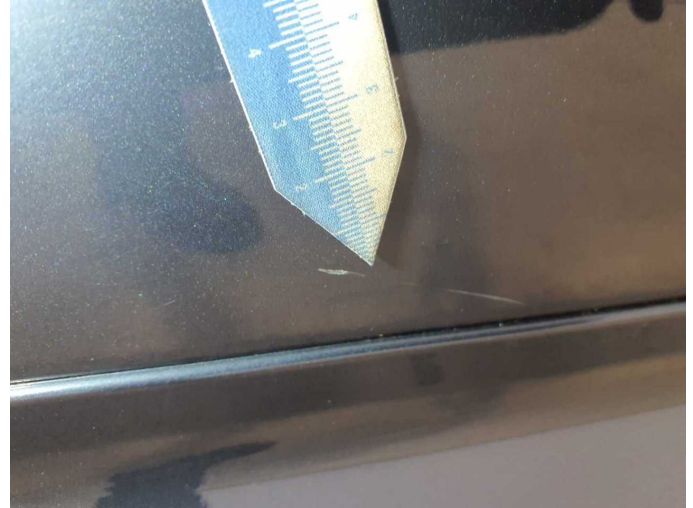
Damage 8: Door - rear right side: Door (Anätzung) - Paint defect - Repair and paint
