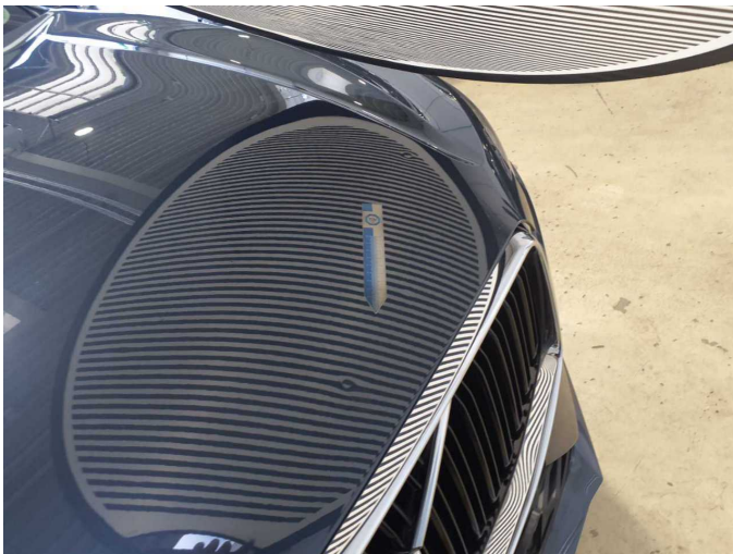
Damage 4: Bonnet: Bonnet - dent(s) - Smooth repair work
