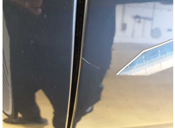
Damage 6: Side panel - rear left side: Side panel - Scratch(es) - Paint
