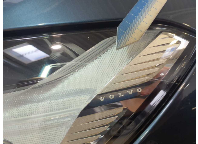
Damage 10: Headlight: Headlight - left side - Scratch(es) - Replace
