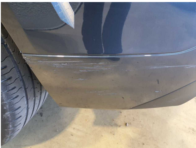
Damage 11: Rear bumper: Rear bumper (Inklusive anbauteile) - Deformed - Replace
