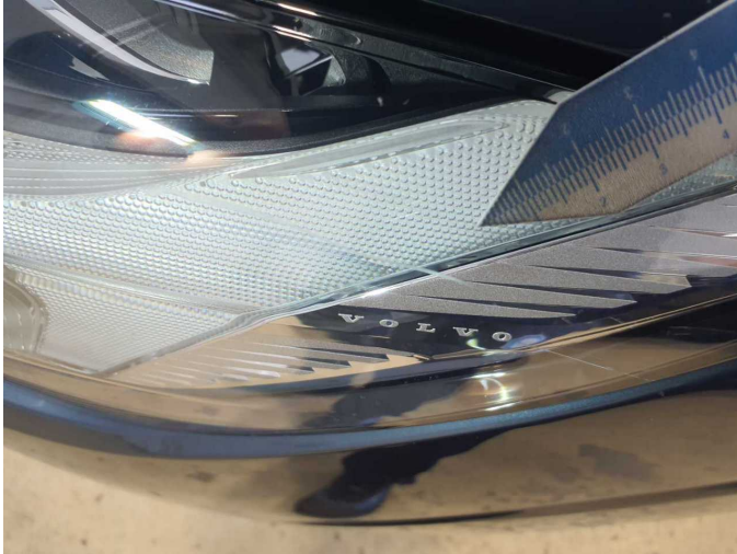
Damage 10: Headlight: Headlight - left side - Scratch(es) - Replace
