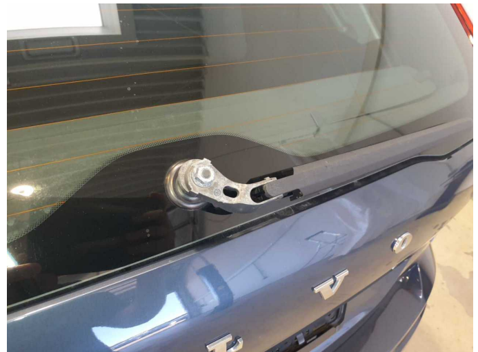
Damage 1: Screen cleaning: Wiper arm - rear (Kappe) - Missing - Replace
