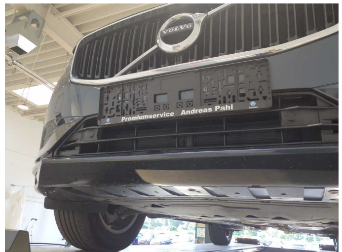
Damage 3: Front bumper: Air-inlet grille - Loose - Repair
