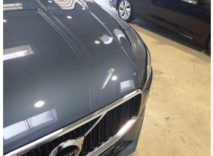
Damage 4: Bonnet: Bonnet - dent(s) - Smooth repair work
