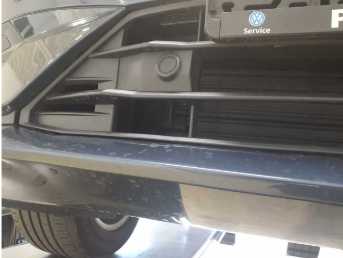
Damage 3: Front bumper: Air-inlet grille - Loose - Repair
