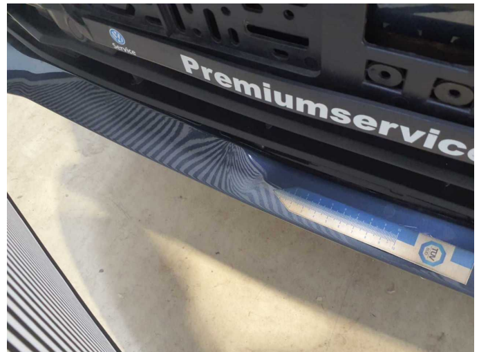
Damage 9: Front bumper: Front bumper - Deformed - Replace
