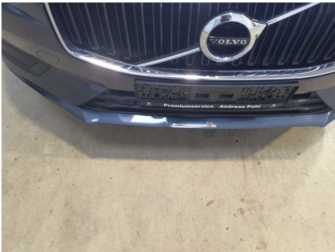
Damage 9: Front bumper: Front bumper - Deformed - Replace
