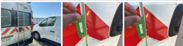
Rear light L, Crack, Replace
