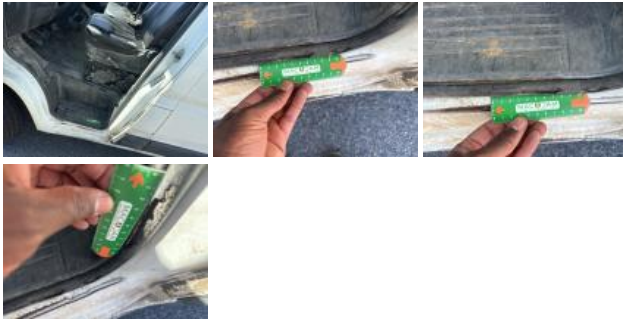
Inner door sill FL, Scratch(es), Paint
