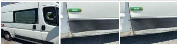
Side panel moulding R, Deformed / Strained, Replace
