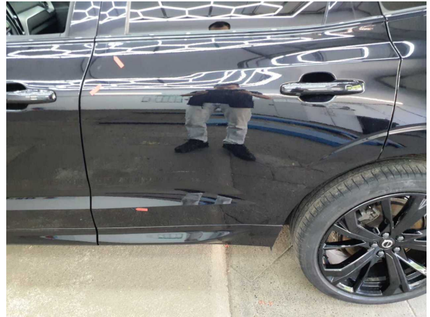
Beschädigung #7: Tür hinten links: Tür - Kratzer - Smart Repair
