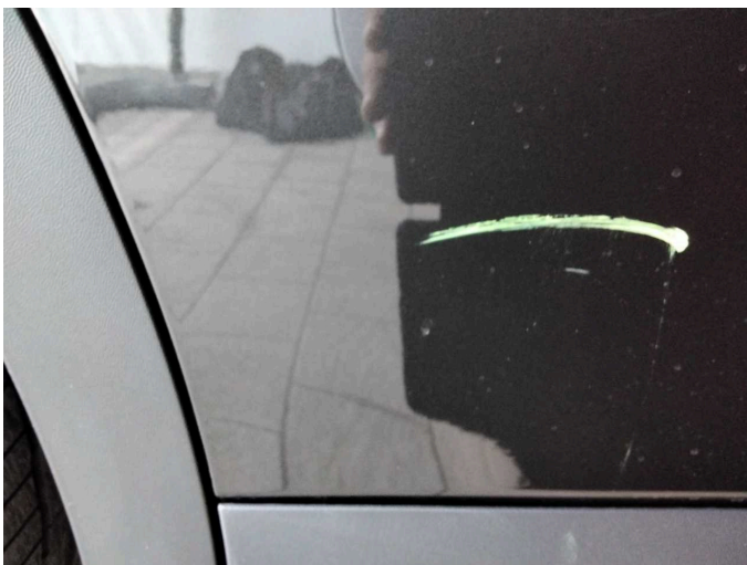
Damage 3: Door - rear right side: Door - Dent / paintcoat damage - Smart repair
