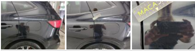
Door FL, Scratch(es), Repair and paint (complete)
