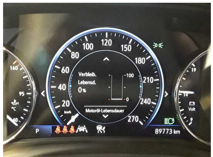
Damage 4: Misc.: Inspection / maintenance - Due - Perform
