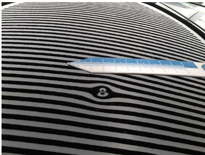
Damage 2: Roof: Roof - dent(s) - Smooth repair work
