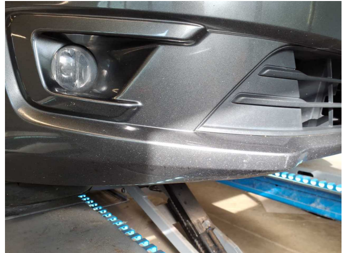
Damage 4: Front bumper: Front bumper (Sandstrahleffekt) - Stone chips - Paint
