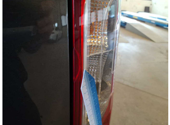
Damage 3: Tail light: Tail lamp - right side - Broken / torn - Replace
