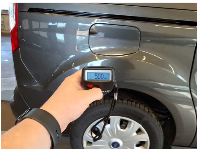
Repainting 1: Boot lid / rear door, Bonnet, Side panel - rear left side, Side panel - rear right side, Door - rear right side, Door - front left side
