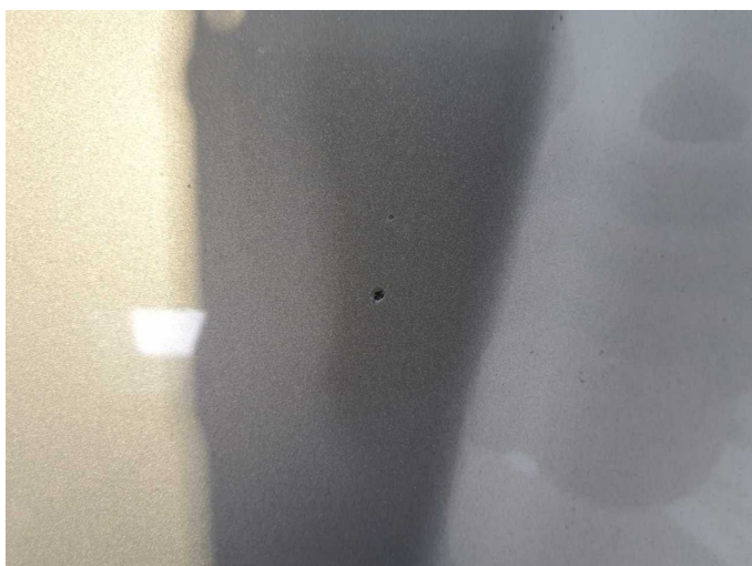
Damage 10: Bonnet: Bonnet - Corrosion - Repair and paint
