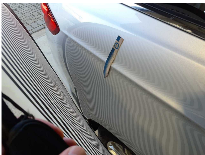
Damage 9: Side panel - rear right side: Side panel (Wellig) - Unprofessionally repaired - Repair and paint
