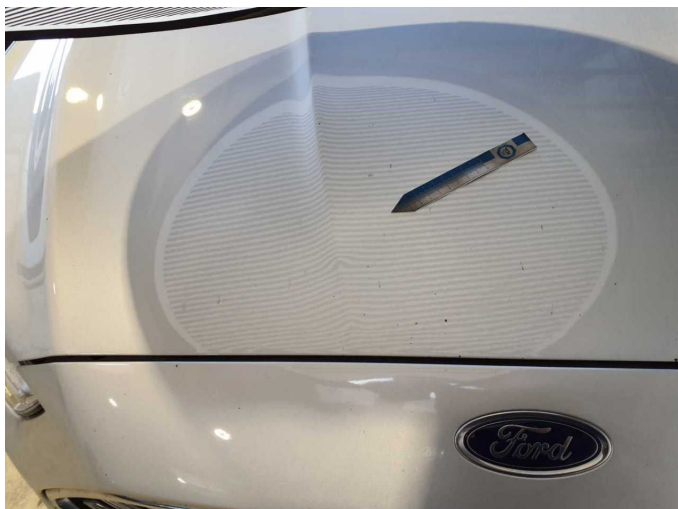
Damage 10: Bonnet: Bonnet - Corrosion - Repair and paint
