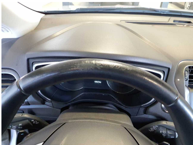
Damage 6: Steering system: Steering wheel - Scratch(es) - Loss in value
