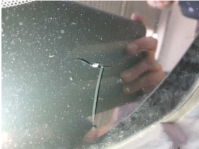
Damage 11: Vehicle glazing: Windscreen - Stone chips - Replace
