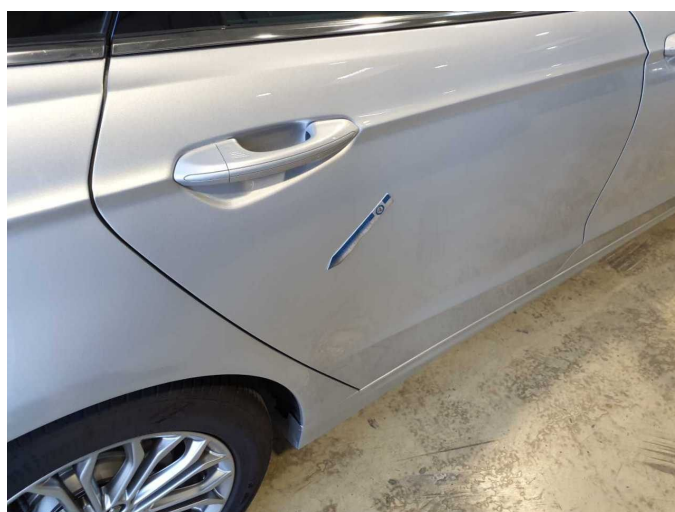
Damage 8: Door - rear right side: Door (Wellig) - Unprofessionally repaired - Repair and paint
