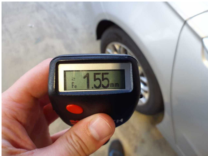
Repainting 1: Side panel - rear right side
