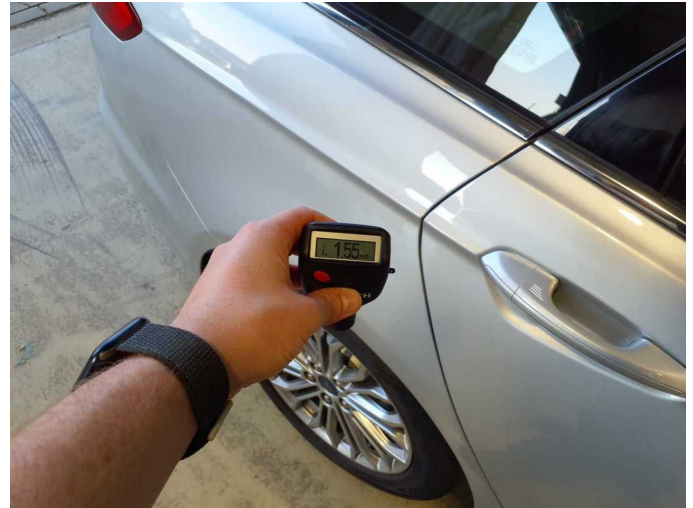
Repainting 1: Side panel - rear right side
