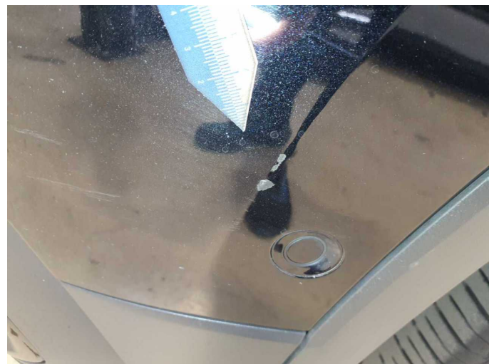
Damage 13: Front bumper: Front bumper - Scratch(es) - Paint
