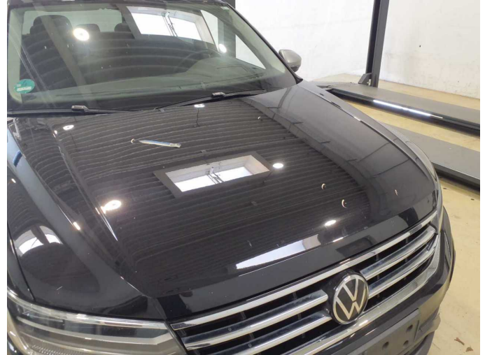
Damage 14: Bonnet: Bonnet - Stone chips - Paint
