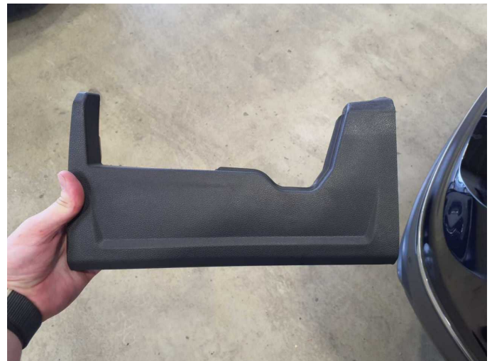
Damage 7: Trim / covers: Trim / covers - Deformed - Replace
