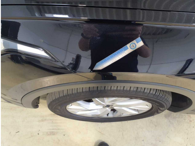
Damage 5: Mudguard - left side: Mudguard - left side - Stone chips - Smart repair
