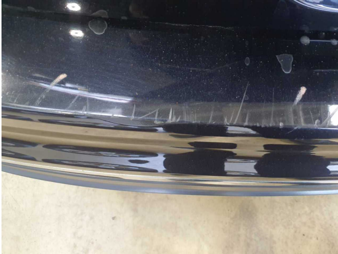
Damage 11: Rear bumper: Rear bumper - Scratch(es) - Paint
