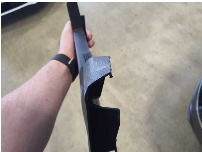
Damage 7: Trim / covers: Trim / covers - Deformed - Replace
