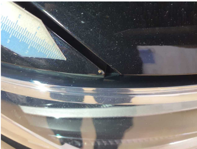
Damage 12: Mudguard - right side: Mudguard - right side - Corrosion - Repair and paint
