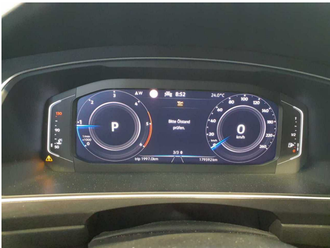
Damage 6: Instrument panel: Indicator light (Ölkontrolle, Ölstand) - on - Perform diagnosis
