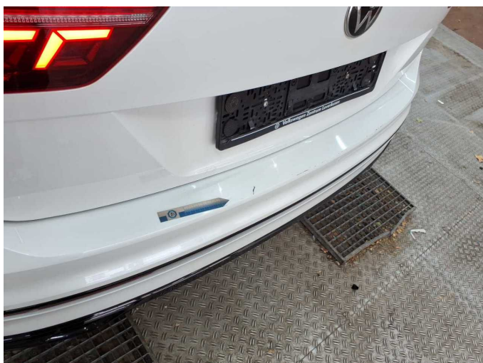
Damage 3: Rear bumper: Rear bumper - Scratch(es) - Paint
