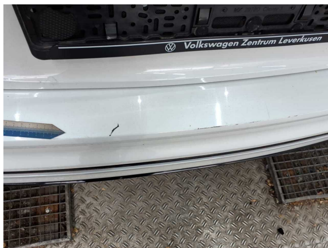
Damage 3: Rear bumper: Rear bumper - Scratch(es) - Paint
