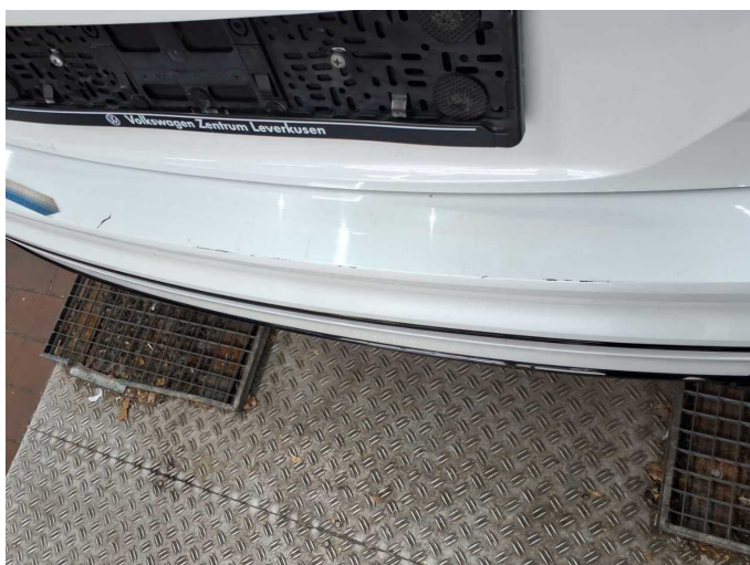
Damage 3: Rear bumper: Rear bumper - Scratch(es) - Paint
