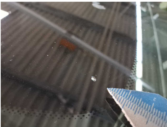
Damage 6: Vehicle glazing: Windscreen - Stone chips - Replace
