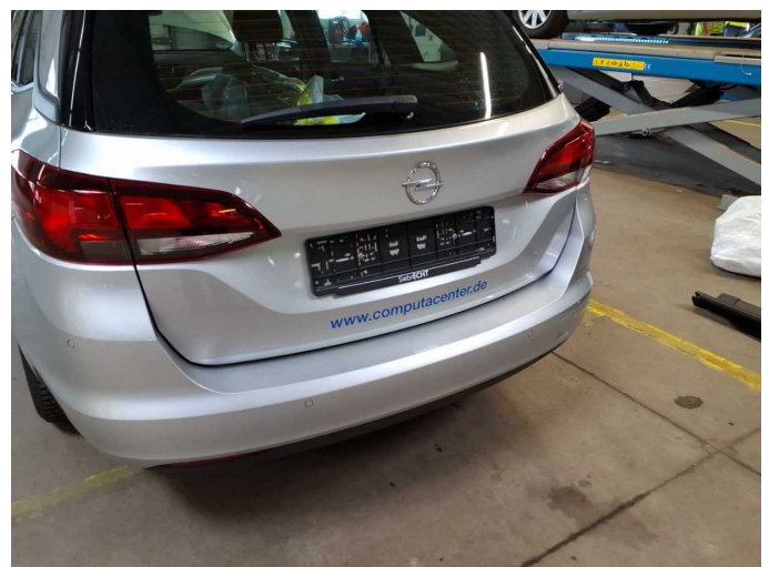
Damage 4: Body: Body - Glued / labelled - De-glug / neutralise
