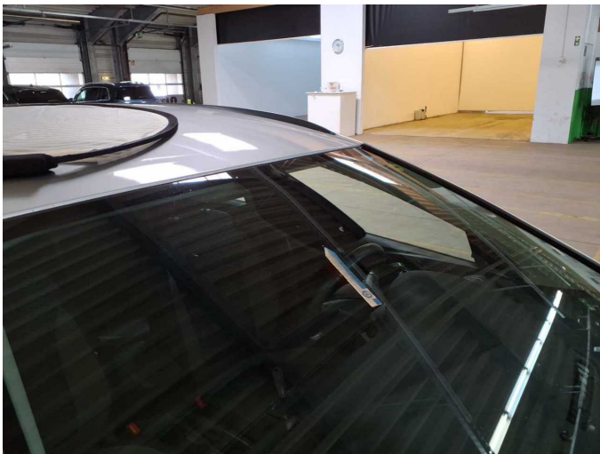
Damage 6: Vehicle glazing: Windscreen - Stone chips - Replace
