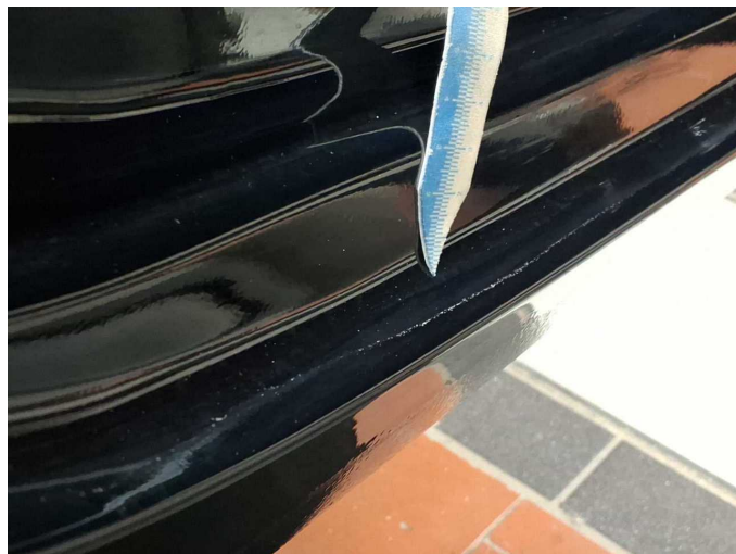
Damage 5: Sill - right side: Sill (Lackläufer) - Unprofessionally repaired - Repair and paint
