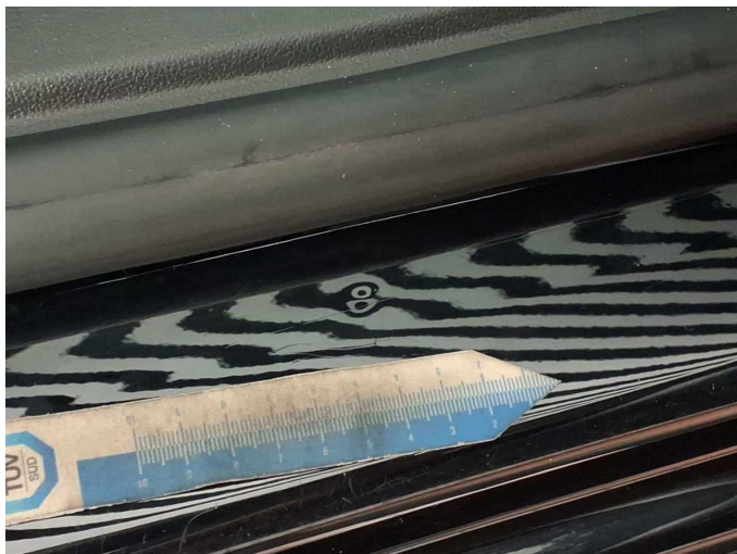
Damage 4: Sill - right side: Sill (+ Kratzer) - dent(s) - Smart repair
