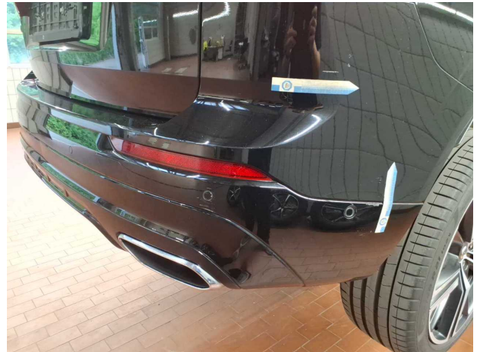
Damage 9: Rear bumper: Rear bumper - Scratched - Paint
