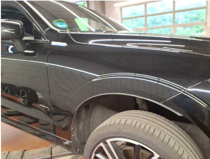
Damage 8: Mudguard - right side: Mudguard - right side - Scratch(es) - Paint
