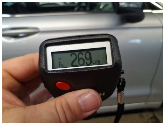
Repainting 10: Door - front right side
