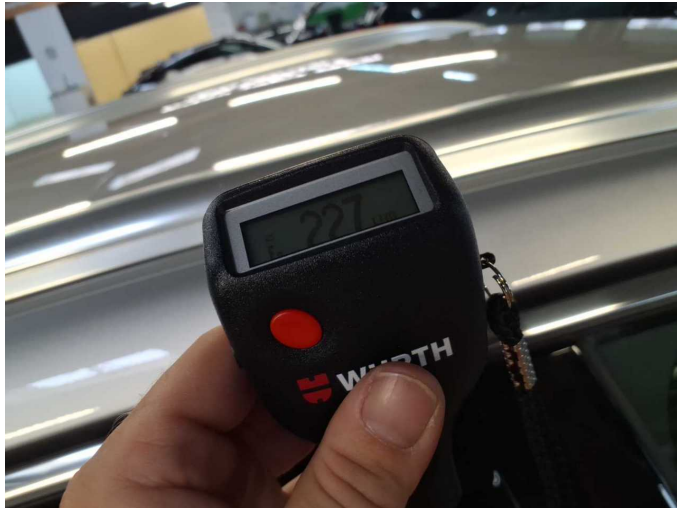
Repainting 2: Roof rail - right side
