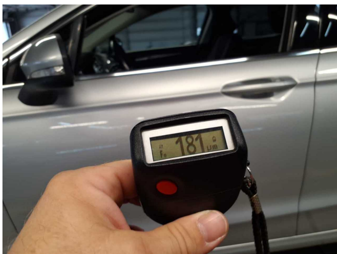
Repainting 9: Door - front left side
