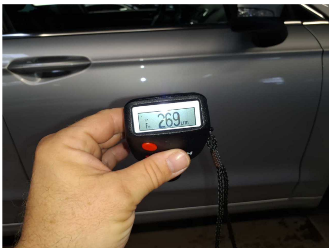
Repainting 10: Door - front right side
