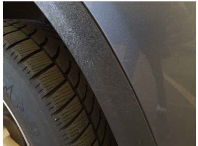
Damage 5: Side panel - rear left side: Wheel well extension - Scratch(es) - Replace
