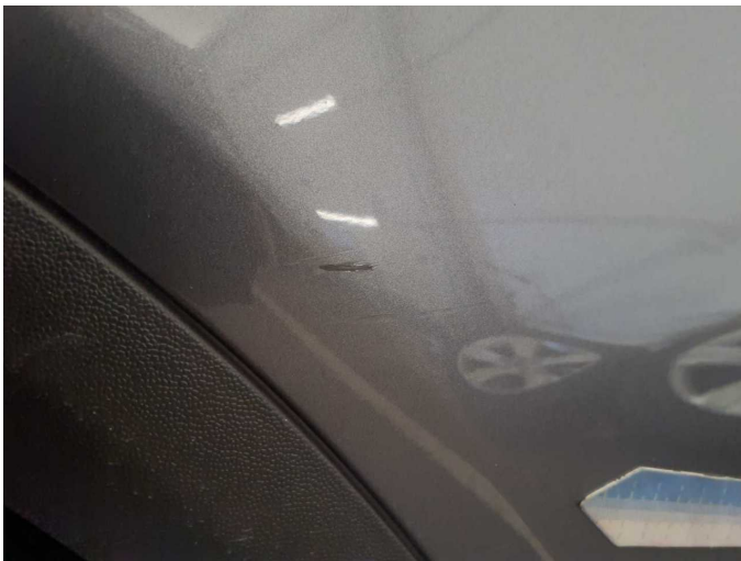
Damage 7: Rear bumper: Rear bumper - Scratch(es) - Paint
