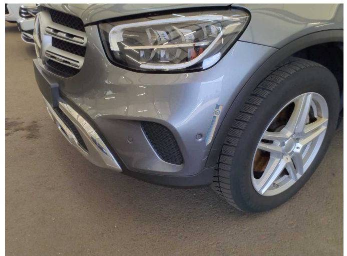
Damage 8: Front bumper: Front bumper - Scratch(es) - repair according to calculation
