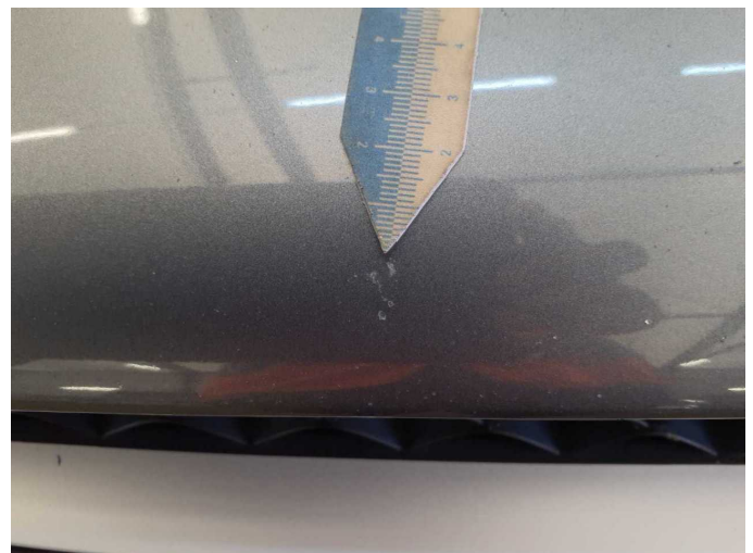
Damage 3: Bonnet: Bonnet - Dent / paintcoat damage - Smart repair
