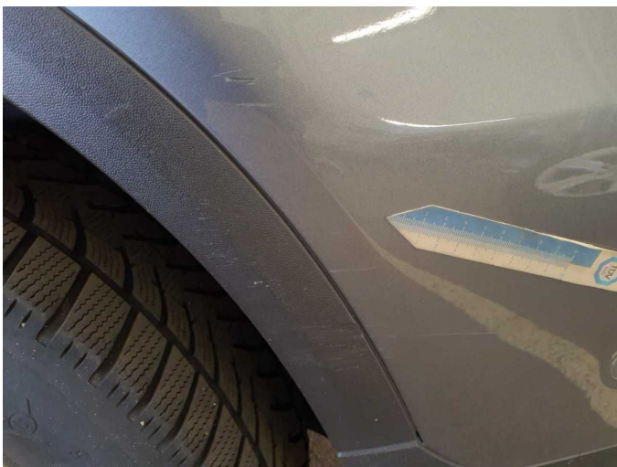
Damage 7: Rear bumper: Rear bumper - Scratch(es) - Paint
