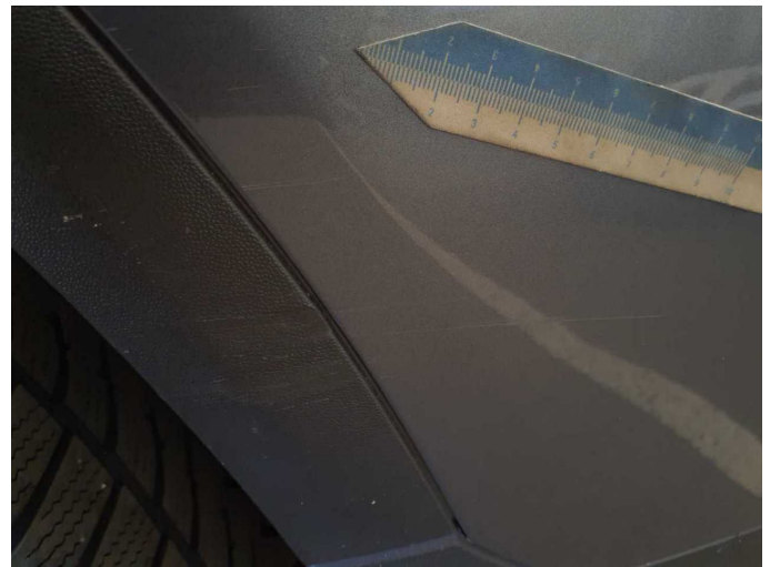
Damage 7: Rear bumper: Rear bumper - Scratch(es) - Paint
