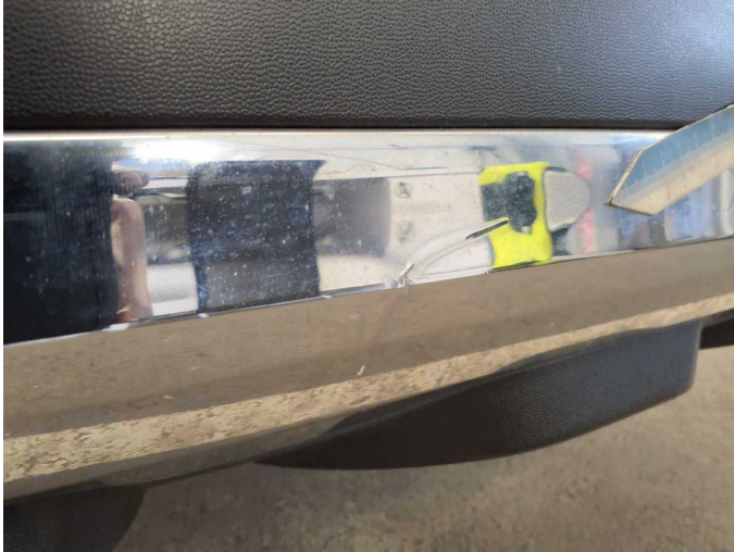
Damage 6: Trim / covers: Brightware / decorative strip - Broken / torn - Replace
